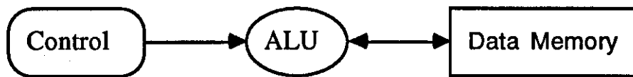
Figure 1.4: The simplest system in Flynn's taxonomy - SISD. Such a system has one control unit and one ALU, with a single instruction stream and a single data stream.
