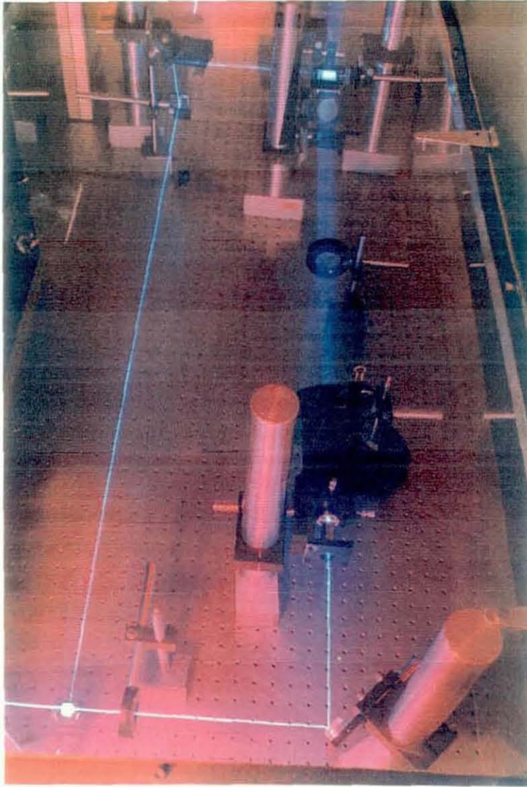
A photograph showing the setup for recording edge-referenced holograms as in Fig. 3.1. The blue area is 458nm light from an argon ion laser. The red light is from a safelight and is used to see the components of the setup.
