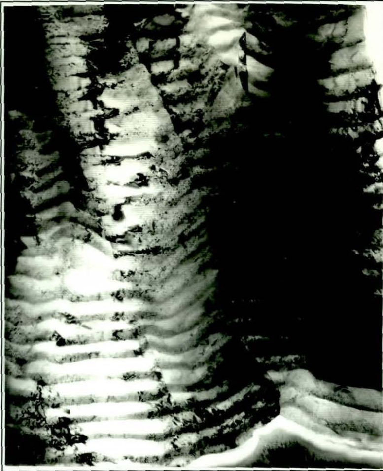
Figure (74). TEM micrograph for 50 layer 25 nm Cu/30 nm Ni CMAM coating
