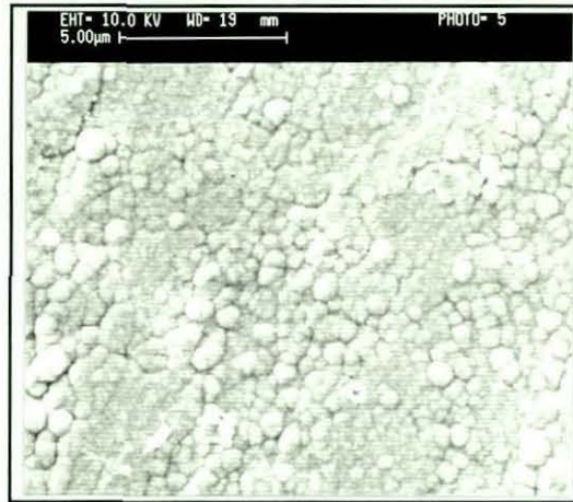
Figure (34). SEM micrograph of an 8 microns thick nickel deposit.
