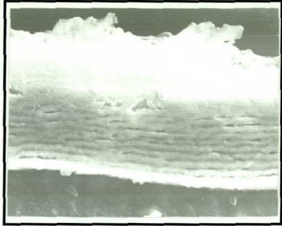
SEM micrograph of 20 layer (40 nm each) Cu/Ni CMAM coating.
