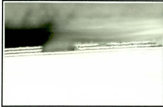
Figure (38) Optical micrograph of a 6 layers Zn/Ni CMMM coating made at different operating conditions (500X magnification)
