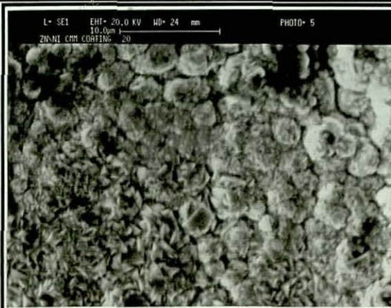
Fig.(119). Surface morphology for 8μ Zn-13%Ni alloy single layer coating
