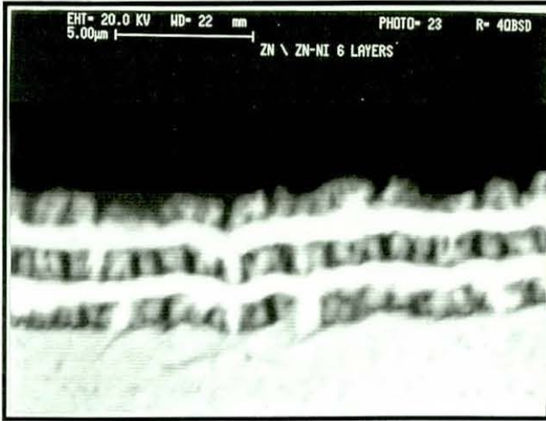
Figure (46A). SEM micrograph for severely etched 8 layer Zn-Ni/Zn and 6 layer Zn/Zn-Ni CMMM coatings
