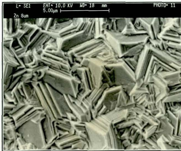
Figure (31). Surface morphology of an 8 micron thick zinc deposit
