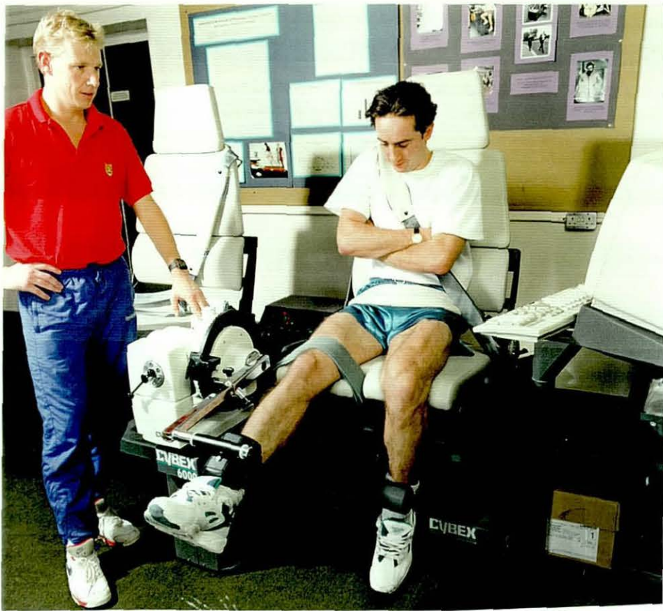
FIGURE 3.3. Subject and equipment placement for testing the knee joint on the Cybex 6000.
