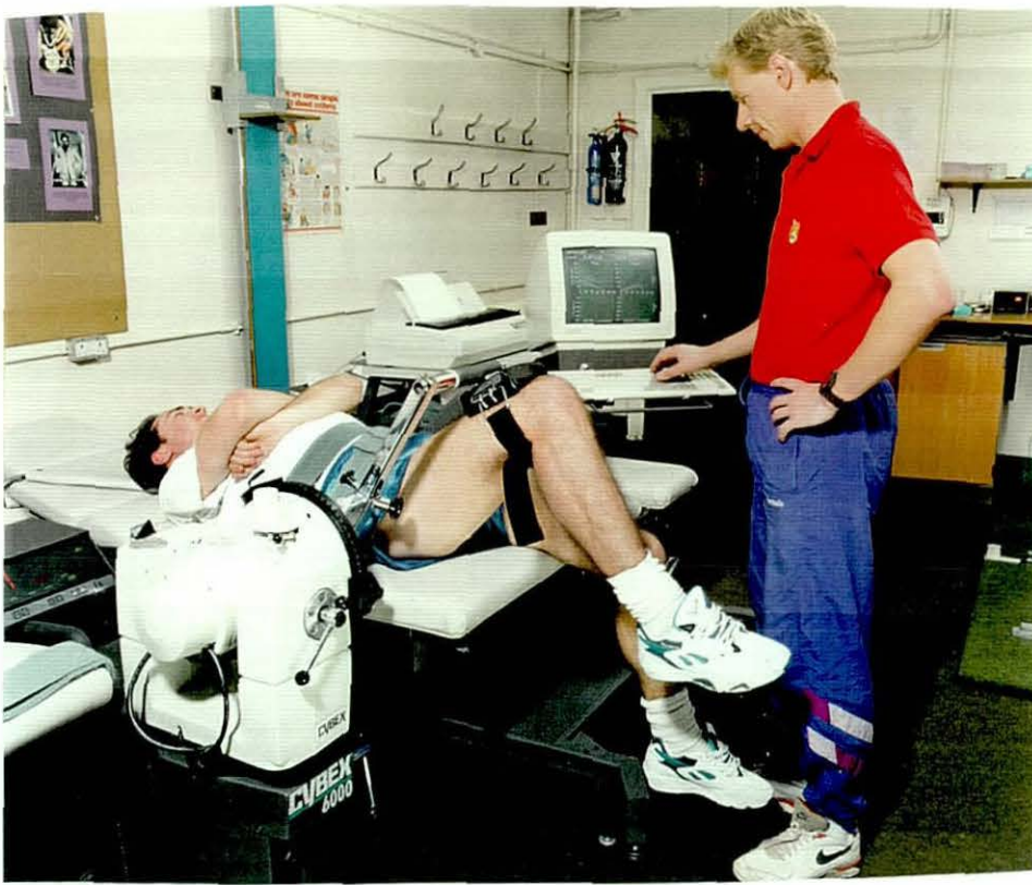
FIGURE 3.4. Subject and equipment placement for testing the hip joint on the Cybex 6000.
