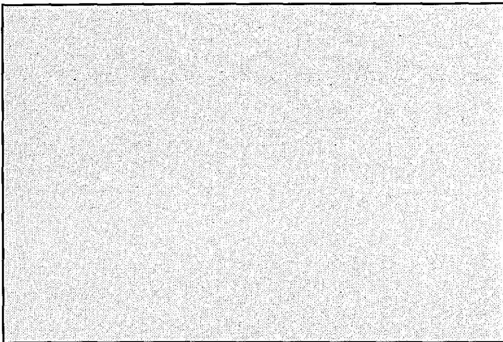
Figure 3.34 - Example of Integrated Image Suffering from Additive Noise. Image taken with X-ray source and image intensifier switched off. Grey levels have been inverted.
