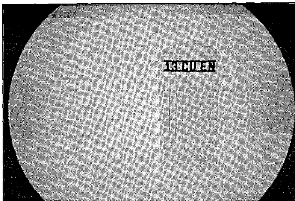
Figure 3.42 - Radioscopic Image of IQI at X-Ray Power Setting 2. Image taken over 300 frames (12 seconds).
