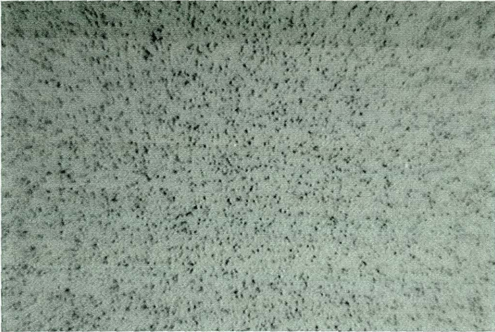
Figure 6.1 - Radioscopic Image of Rubber-Tungsten Sample with No Strain. Image Processed to reduce shading and frequency dependent Noise.
