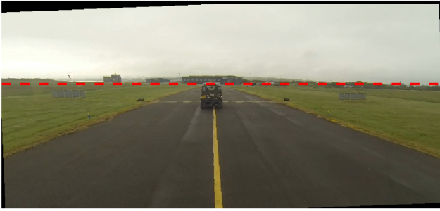
Fig. 6 Stabilised video frame with the reference horizon
