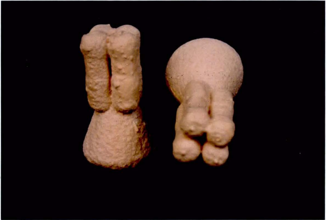
Figure 4.10 : A shell investment mould for casting of tensile test specimens.
