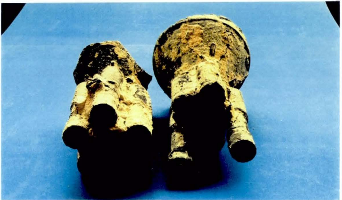
Figure 5.8 : Casting produced in a mould heated to a temperature of 630\text{ }^{\circ}\text{C} \pm 10\text{ }^{\circ}\text{C}
