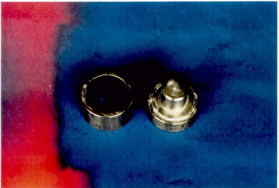
Figure 4.4 : The Shaw process mould
