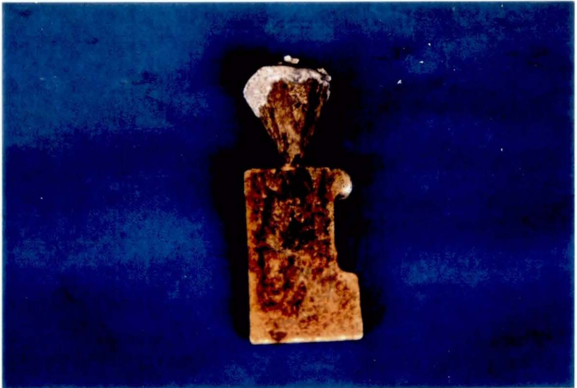
Figure 5.6 : Casting produced in a mould coated with SEMCO mixed with 2% \text{KBF}_4 .
