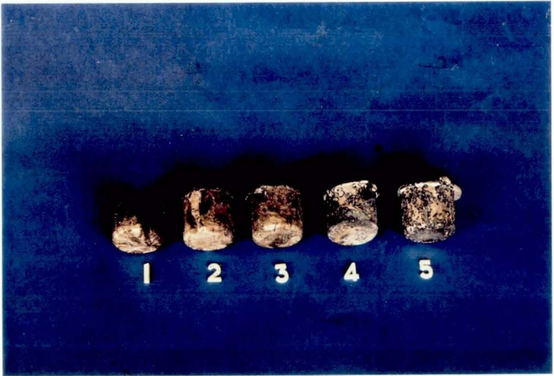
Figure 5.5 : Castings produced using moulds containing various percentages of \text{KBF}_4 :
