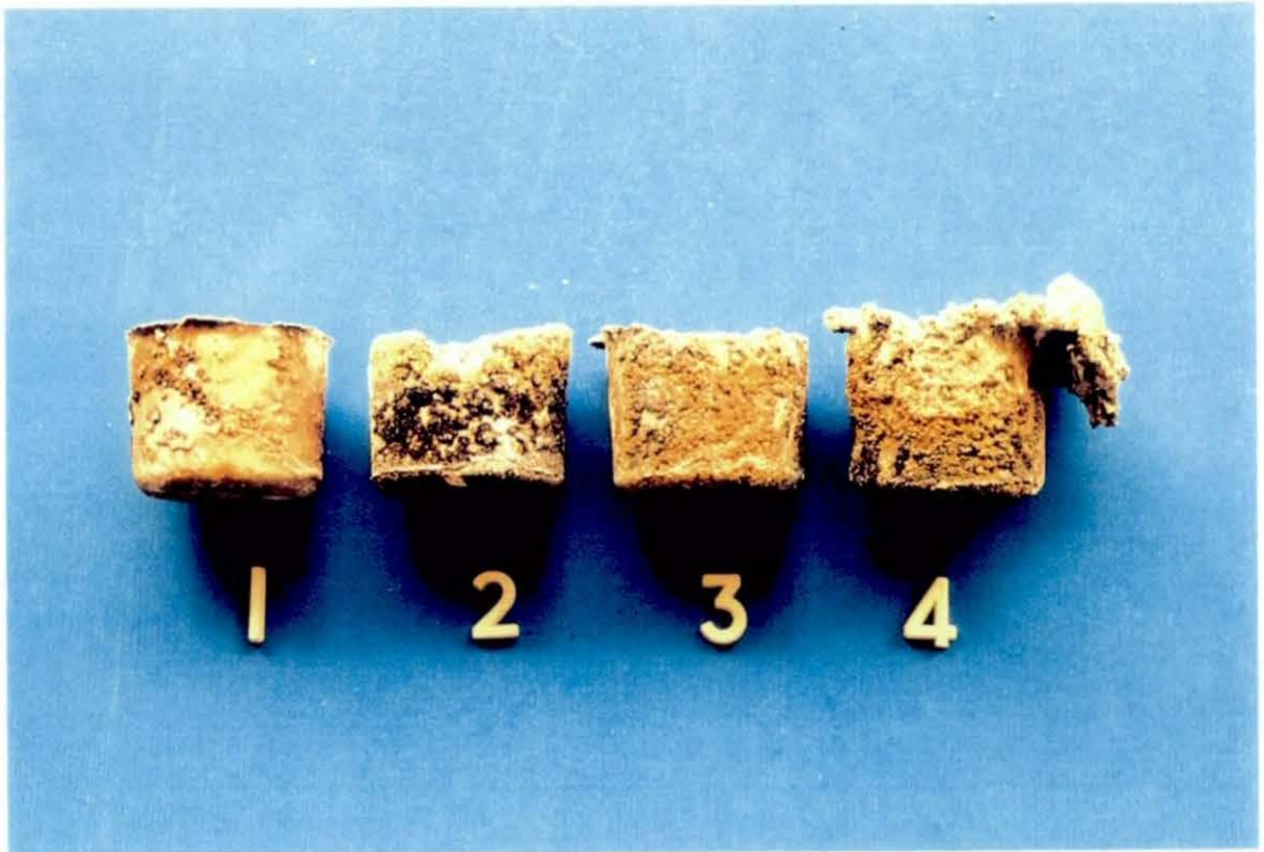
Figure 5.7 : Castings produced in anhydrous calcium sulphate moulds poured at different pouring temperatures : 1) 700°C 2) 730°C 3) 750°C 4) 780°C
