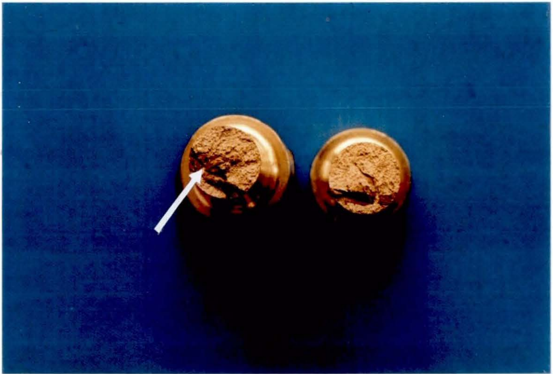
Figure 6.3 : Inclusion on one of the fractured surfaces of a casting produced using flux method melting
