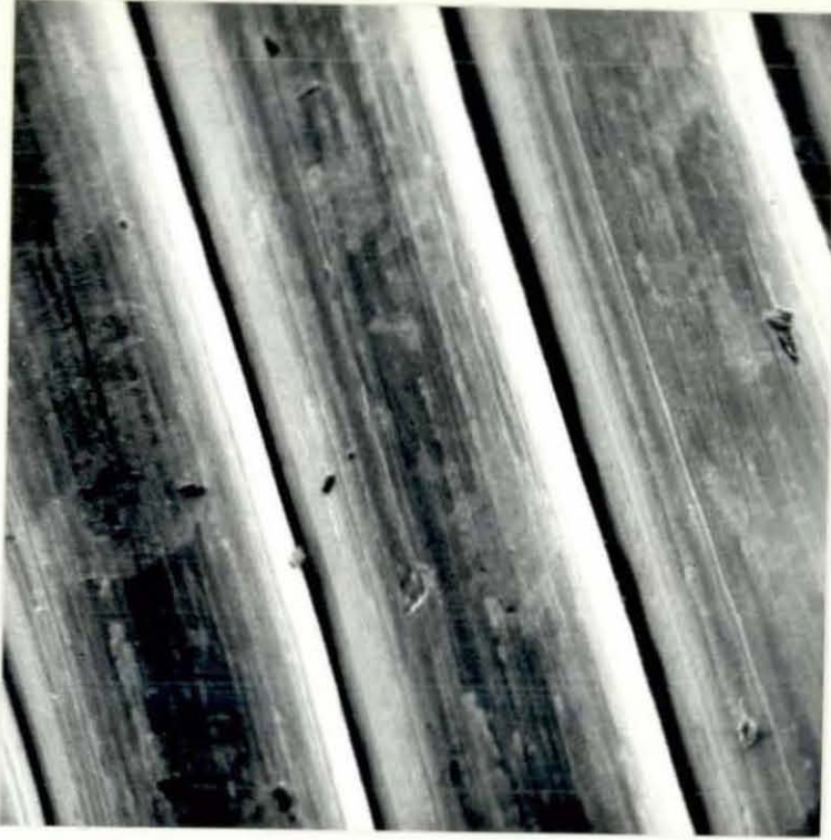
FIGURE 4.6(a) SEM Micrograph of Wire Surface Debonded from the Unfilled SBR. It shows there is no Rubber Bonded to the Wire Surface (Magnification 100)
