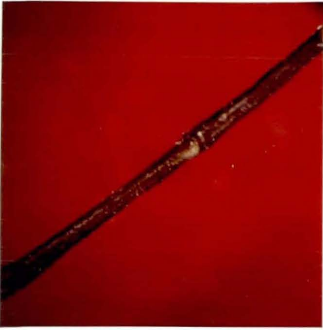
(a) with rubber failure of the adhesive bond
