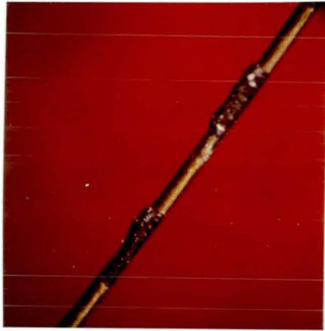
(c) partially with rubber failure and partially interfacial failure
