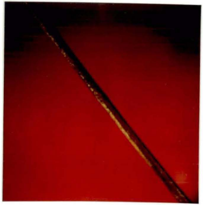
(b) rubber brass interfacial adhesion failure
