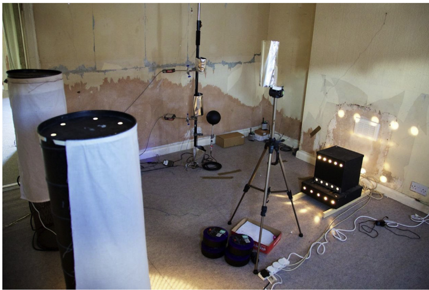
Fig. 3. Synthetic occupancy and monitoring equipment in the living room of the right Test House. The image shows at the back of the room the shielded temperature sensors at three heights and the black globe thermometer. On the left and right of the image there are the custom-made ventilated matt black metal cylinders and boxes used as synthetic occupancy, providing gains for two ‘occupants’, electrical appliances and lights.
