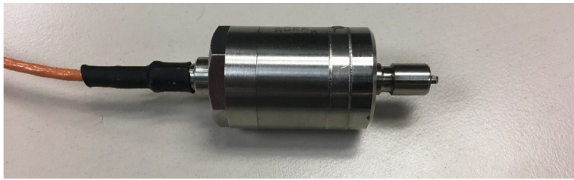
Figure 9.6: DRUCK pressure transducer
