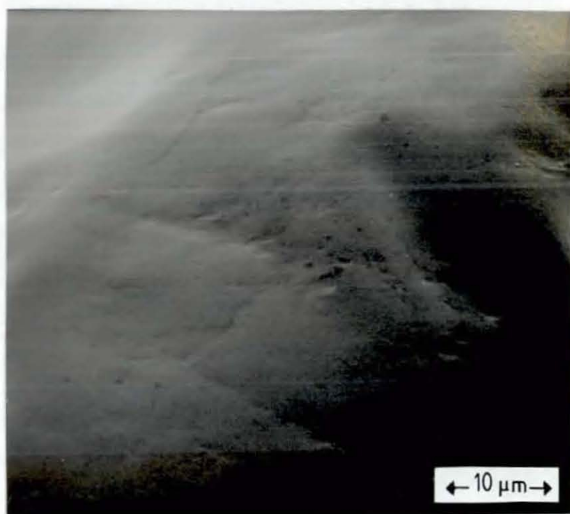
SEM Micrograph of Blend 156 (2000 x) [ melt pressed ]
