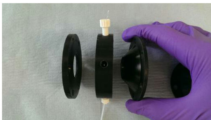
Figure 4.5 - Side profile showing front cover A1, main body A2 and middle conical part A3 / A4
