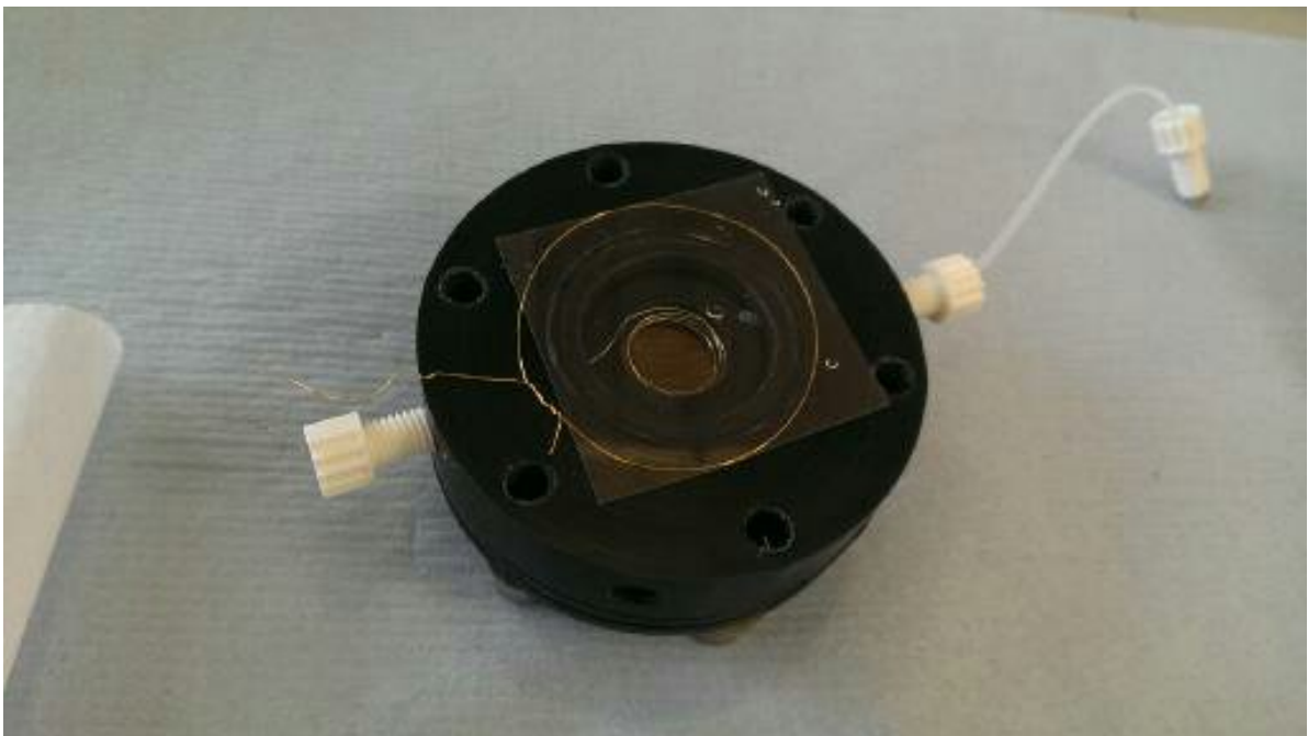
Figure 4.8 - Installation of front working electrode E, gold wire D placed between cell body A2 and ITO polyester film, gasket M and front cover A1 to be installed (not shown) O ring L positioned in cell body
