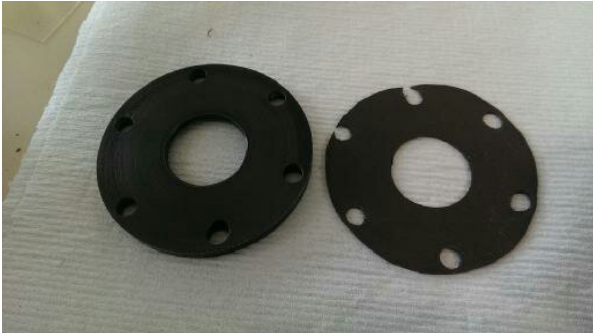
Figure 4.9 - (Left) front cover A1 (Right) neoprene gasket M
