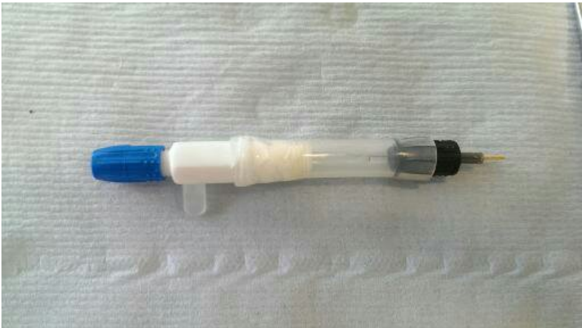
Figure 4.10 - Reference electrode setup, to be connected to luggin capillary H via connection port.
