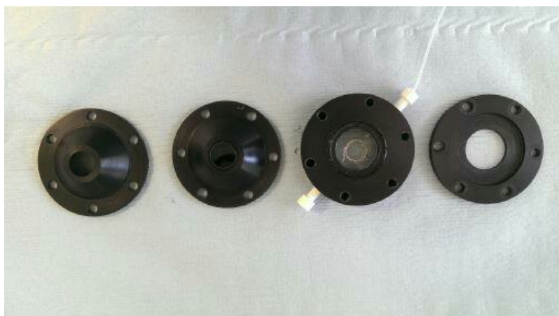
Figure 4.3 - (Left to right) rear conical part A4, middle conical part A3, main body A2, front cover A1
