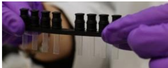
Figure 26: MCF strips, each 3cm in length in the rubber connector strip (Capillary Film Technology 2014).
