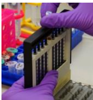
Figure 28: Turning of the MSA knob while the MCF strips are inserted into reagent wells (Capillary Film Technology 2014).
