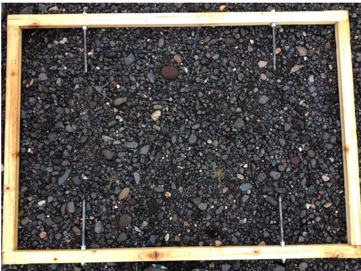
Figure 3.6: Automated sediment sizing using technique described in Graham et al., (2005a, 2005b)
