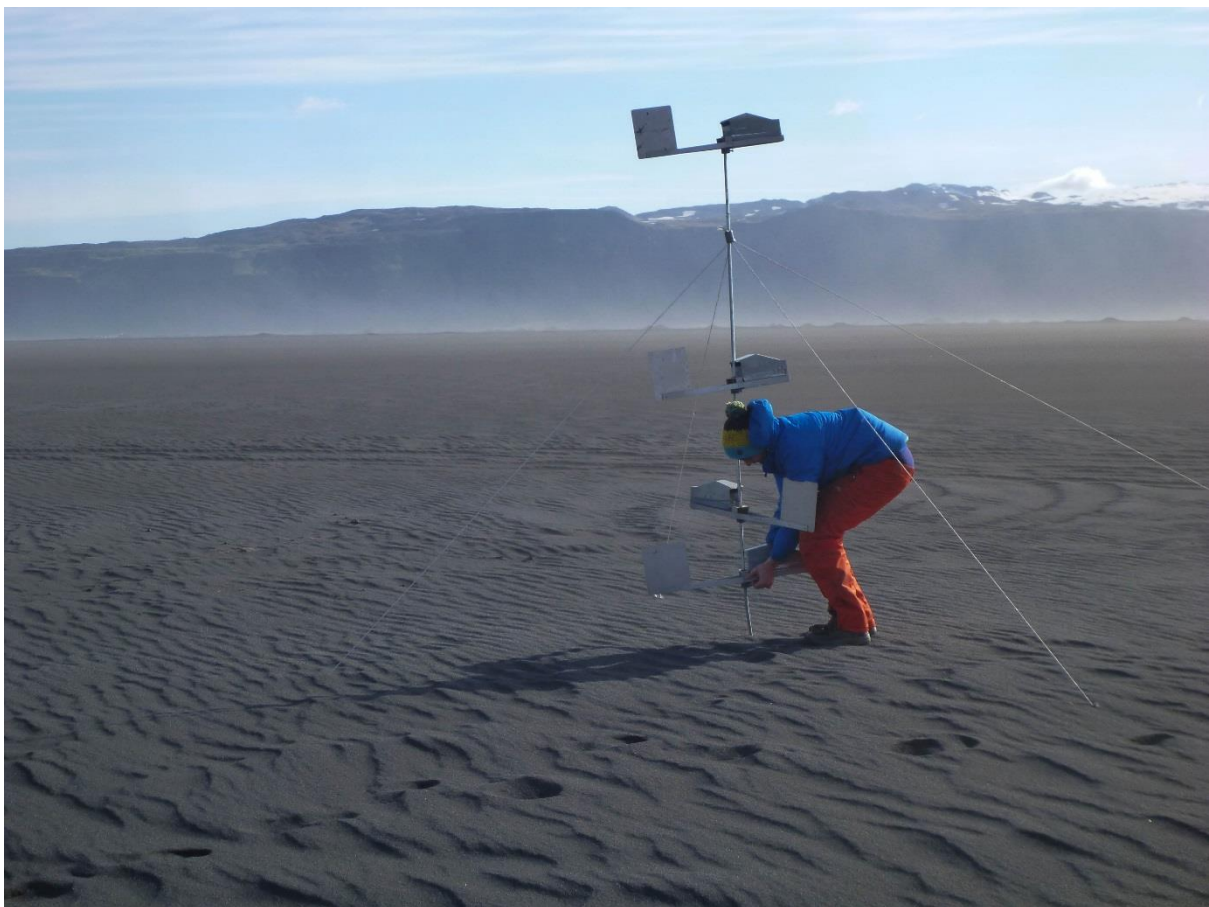
Figure 3.4: Monitoring wind erosion using BSNE Traps on the relict sandur system at Markarfjot (June 2015)
