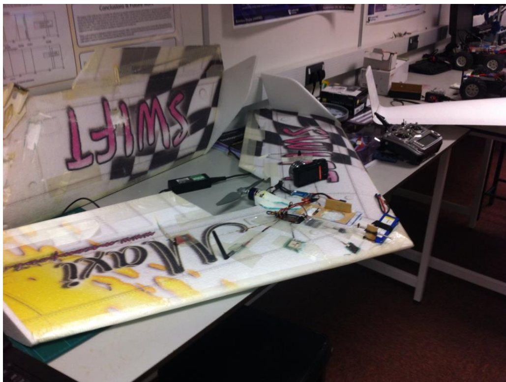
Figure 3.2: Loughborough University Delta Fixed Wing Unmanned Aerial Vehicle
