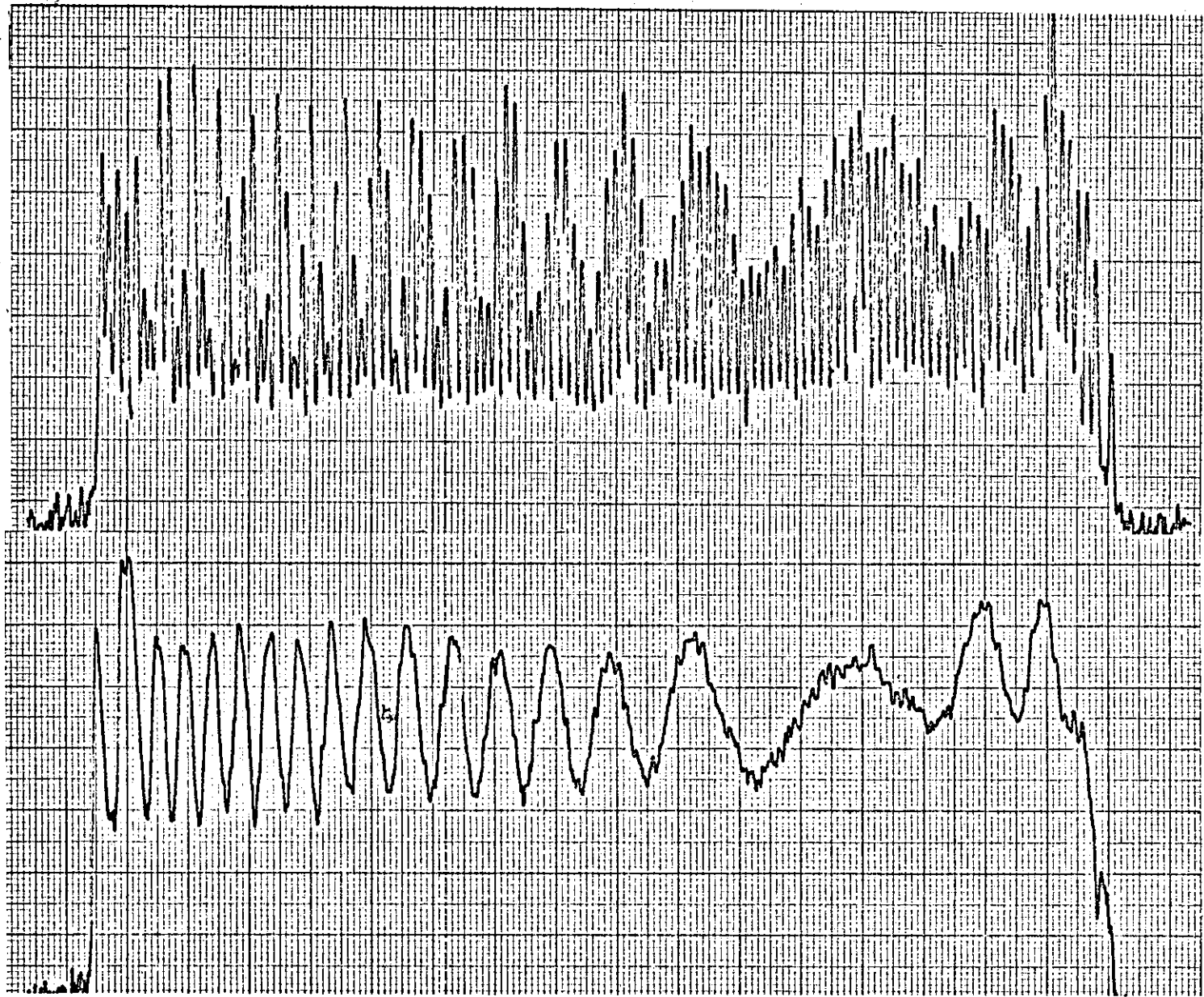
FIG. 14. MICRODENSITOMETER TRACES ACROSS A NEGATIVE OF A CONTOURED TURBINE BLADE (MOIRÉ SHADOW CONTOURS).
