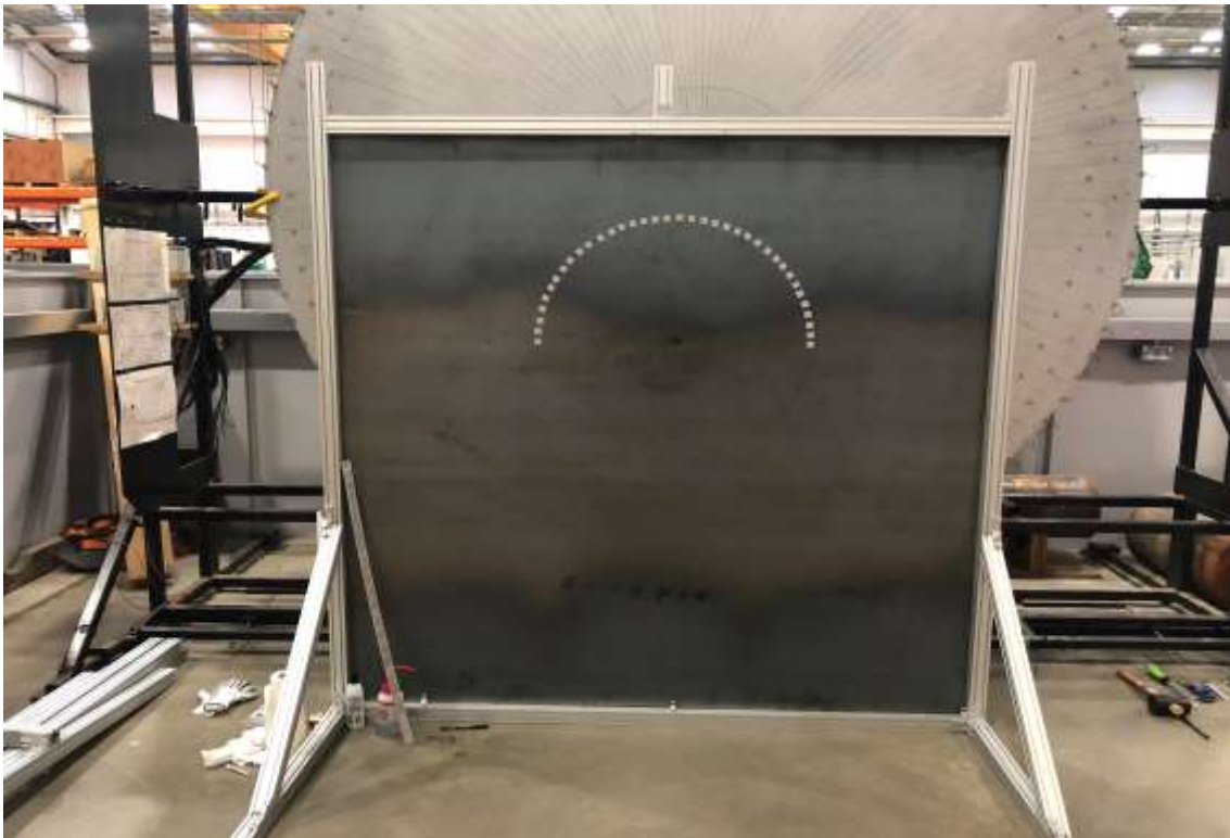
Figure 4 Picture of the waveguide used for vibrometry studies, 2x2x0.003 m steel plate
