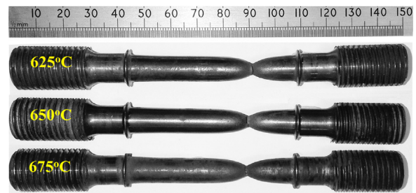
Fig. 4. MarBN specimens after creep testing showing necking.
