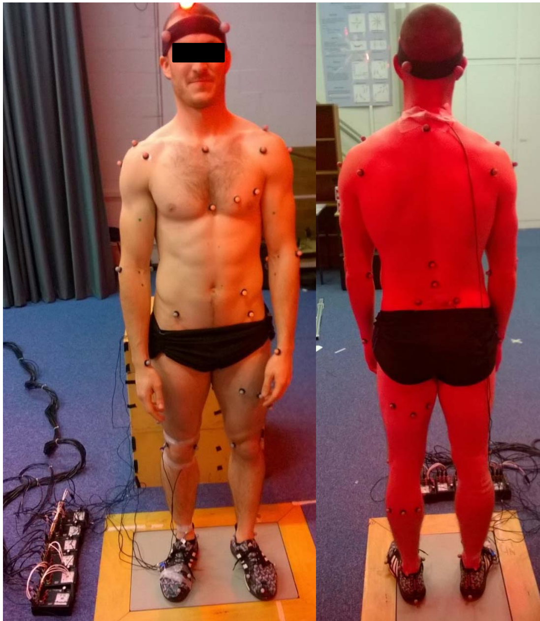
Figure 3.3 Positioning of reflective markers on the subject
