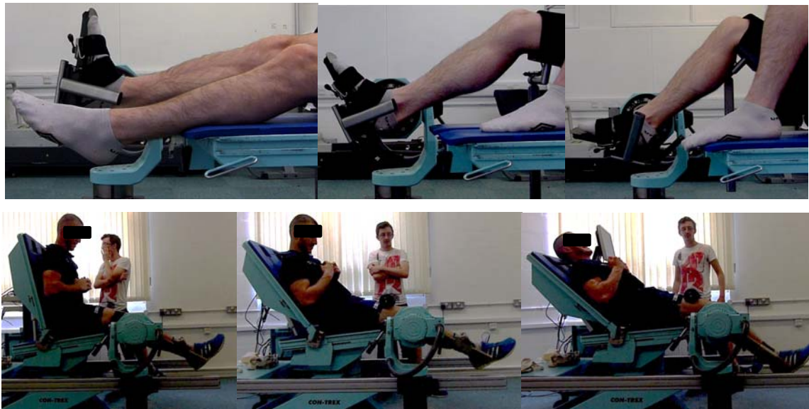
Figure 6.2. Isovelocity dynamometer configuration at three secondary joint angles each for ankle plantarflexion (top); and knee flexion and extension (bottom).
