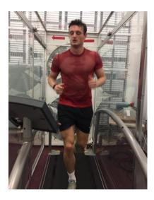
**Figure 3** Participant running on the treadmill located into the wind tunnel which was placed in the environmental chamber.
