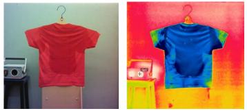
**Figure 2** Digital and Infrared pictures of identical views for front and back of the T-Shirt, including black body calibrator positioned on a stool behind the T-Shirt stand.
