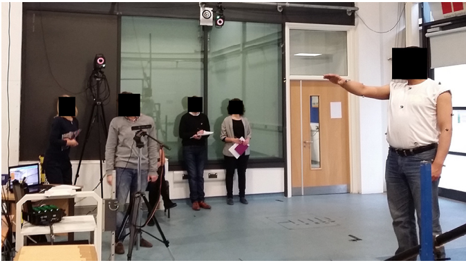
Figure 2 Study set-up showing motion capture cameras, Medical Interactive Recovery Assistant (MIRA) software (MIRA Rehab Ltd., London, UK)/Kinect (Microsoft Corp., Redmond, WA, USA) sensor, and trained observers.
