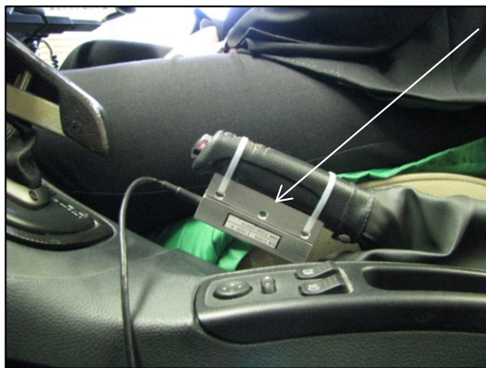
Figure 8.4 Load cell fixed to parking brake lever
