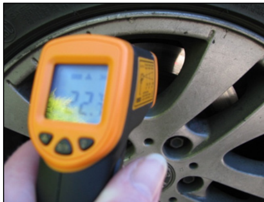
Figure 9.5 Recording rear brake temperature with an infrared pyrometer
