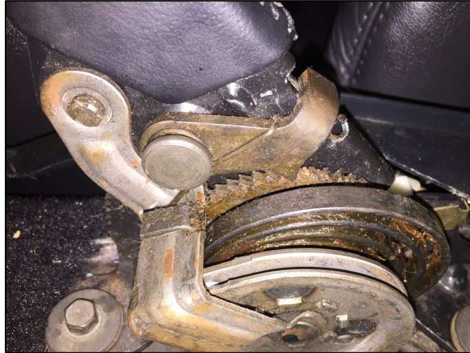
Figure 3.10 Parking brake lever ratchet and pawl
