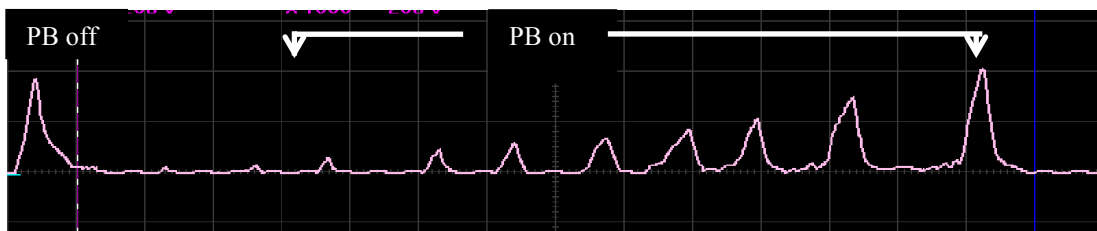
Figure 8.27 Force applied when the parking brake lever is pulled up ratchet by ratchet (20% gradient)
