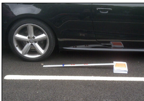
Figure 8.19 Measuring the gradient
