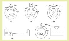
Figure 2.1: Types of Keys: (a) Square key, (b) Rectangular key, (c) Kennedy key, (d) Gib-head key, and (e) Woodruff key.
