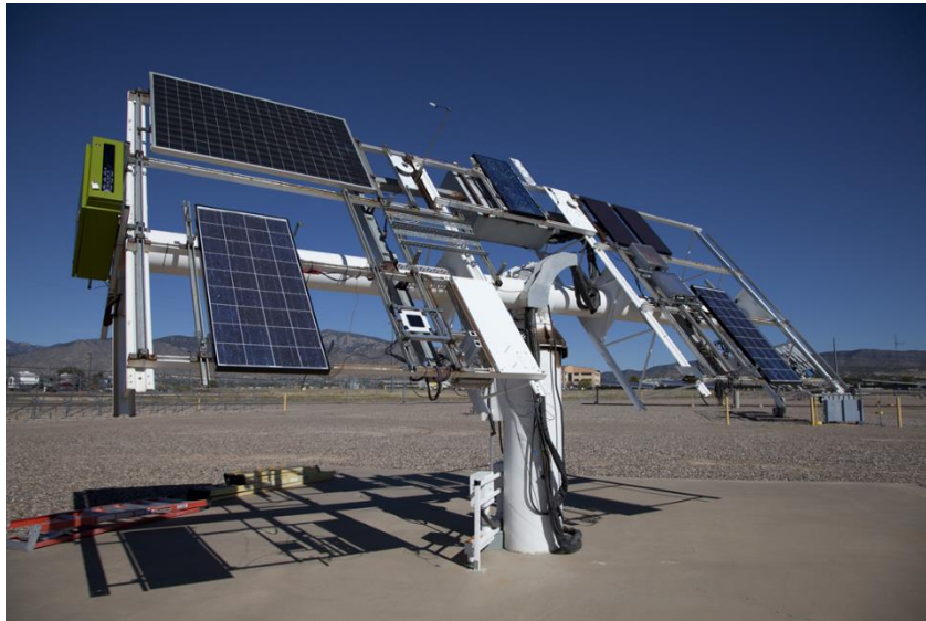
Figure 5. 3. Photograph of two-axis tracker for outdoor angular response characterisation of PV modules as used by Sandia National Laboratories [95].
