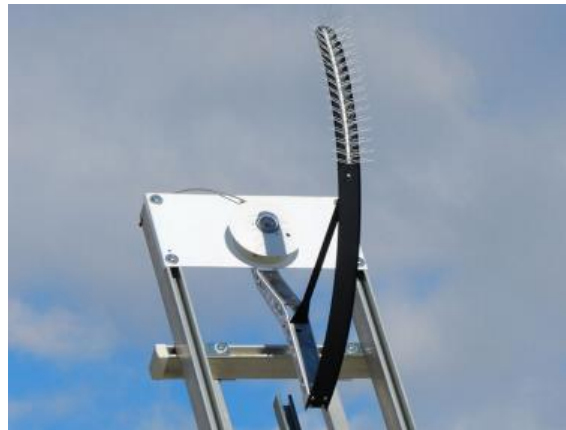
Figure 5. 4. Photograph of pyranometer with diffuser attachment for the measurement of diffuse in-plane irradiance reported in [82].
