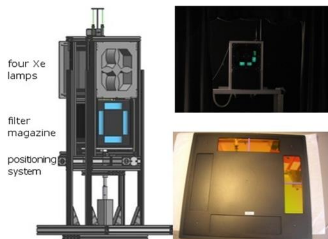
Figure 3. 2. Figures showing the SR measurement setup using pulse light solar simulator with interference filter (left) and photograph of a unit of filter as used in SUPSI (right) [56].
