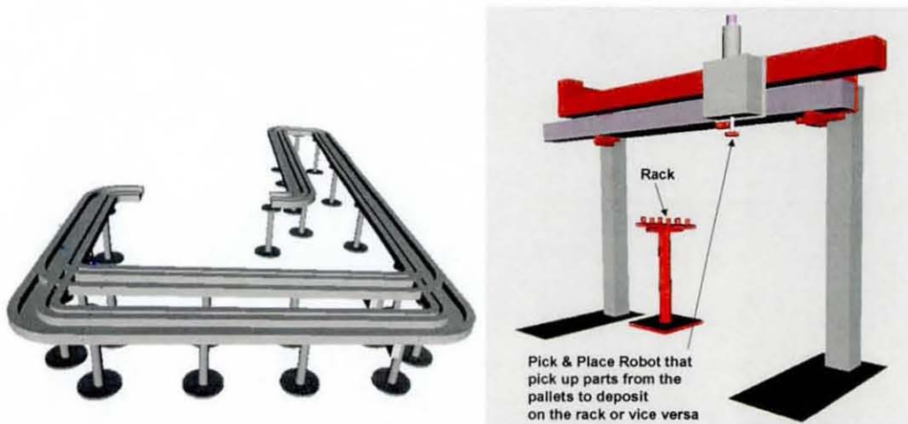
Figure 7.25 A 3D VRML model of the Krause test machine. Left: transport system which is a conveyor. Right: assembly system consisting of the pick-and-place station
