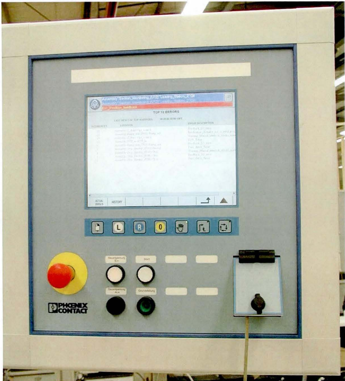
Figure 7.14 Implemented HMI Console on J.A. Krause Case Study demonstration machine
