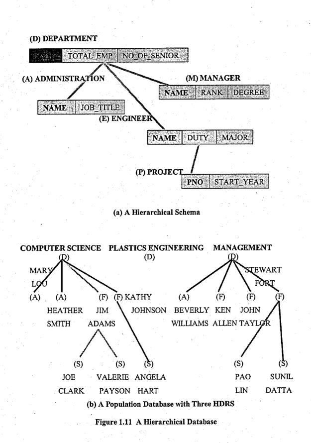
Hierarchical databases have their idiosyncrasies. They can be useful for some applications, i.e. the functional mapping between parent and children and the hierarchical structure, whereas others pose restrictions. To be specific, in a hierarchical or tree data structure, there is "many-to-one" mapping (which include one-to-one) from children nodes (records-type instances) to the root instance.
