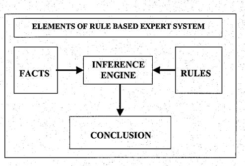
Figure 5.1 Basic Elements of Rule-Based Expert System
