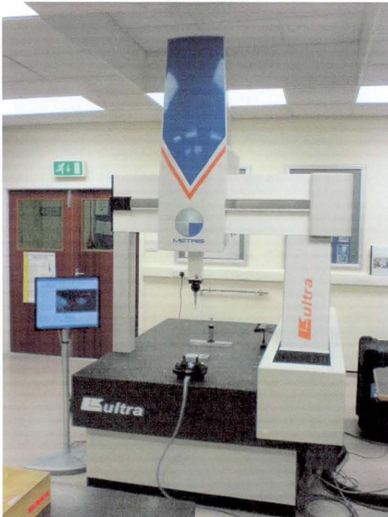
**Figure 1-4: A mechanical CMM with a bridge structure.**
