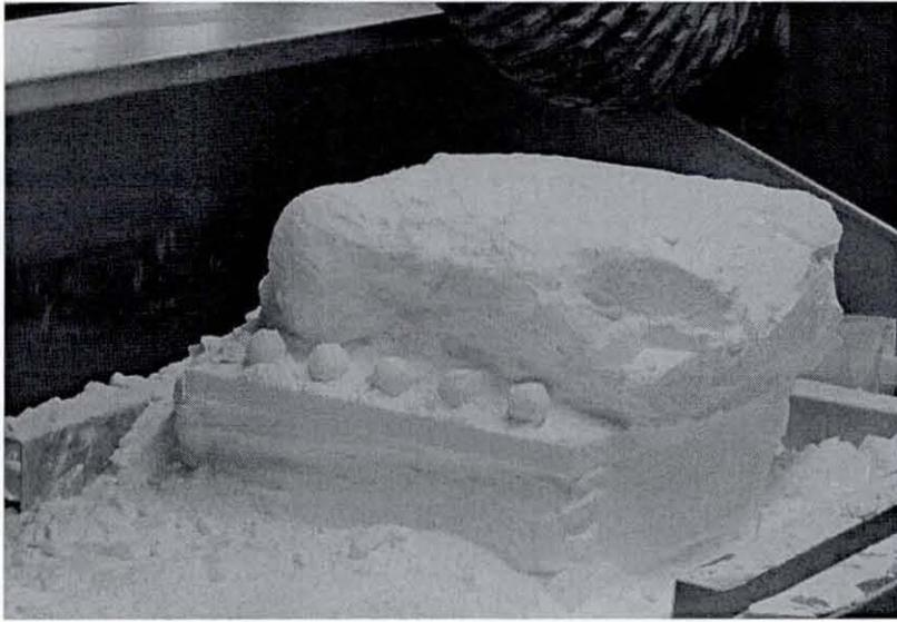
Figure 4-4: Artefact covered with powder on leaving the SLS machine.
