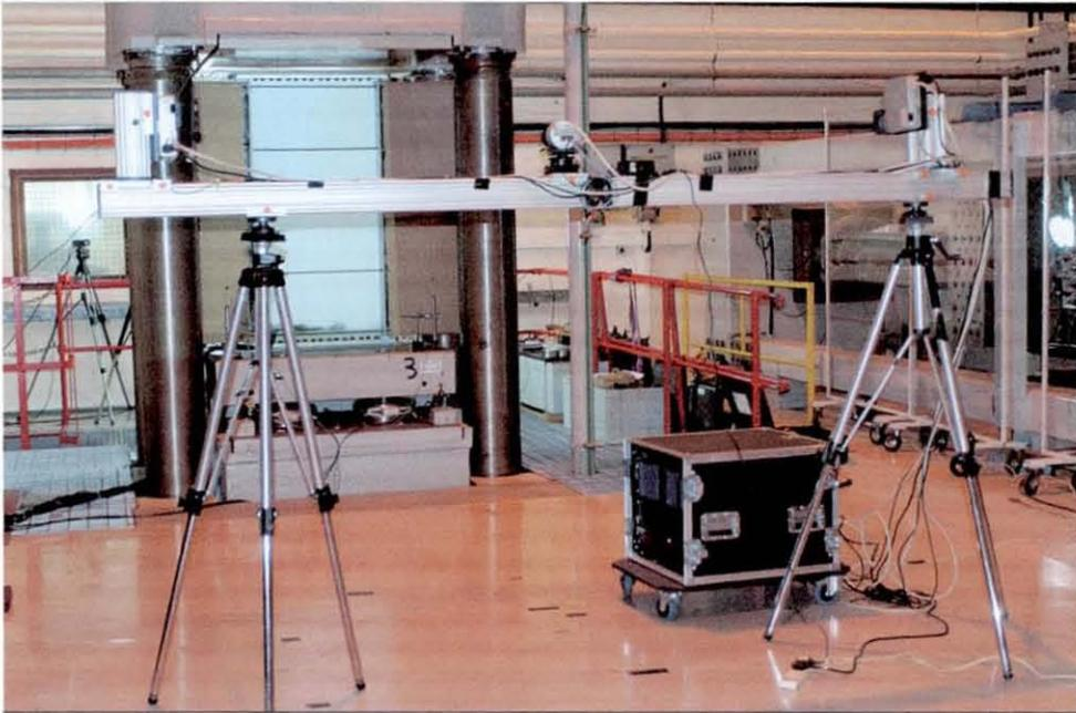
**Figure 8-2: One-camera two-projector optical SMS facing a compression panel positioned in a test rig at Airbus' Bristol site.**
