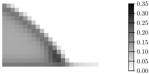
Figure 7.12: Magnification of a portion of the time t = 2.98 \times 10^4 nanoparticle density profile in Fig. 7.11, in the contact line region.
