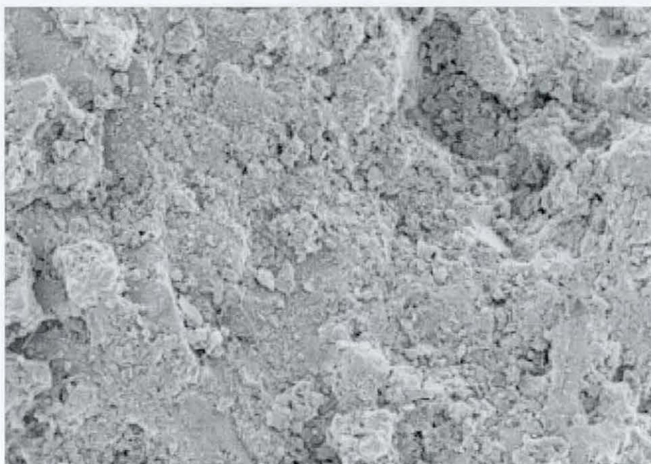
Figure 6.23 SEM image of \text{Ni}/\text{ZrO}_2/\gamma\text{-Al}_2\text{O}_3 catalyst, effect of \text{NH}_3 for 6 hours, \text{WHSV} = 19200\text{ml/hr g cat}
