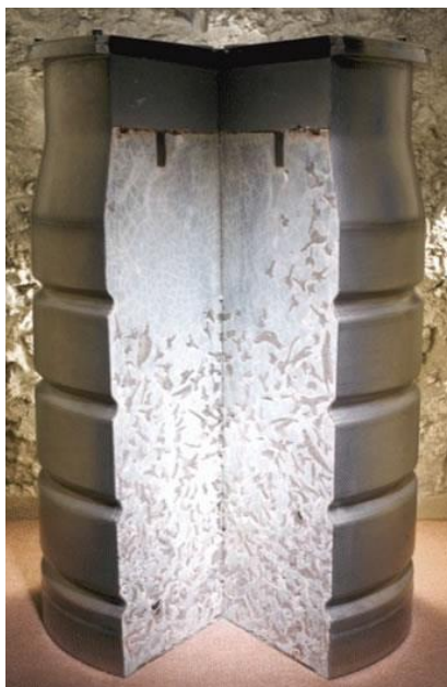
Figure 1.12 - Cross-section of a filled barrel proposed for the GDF
