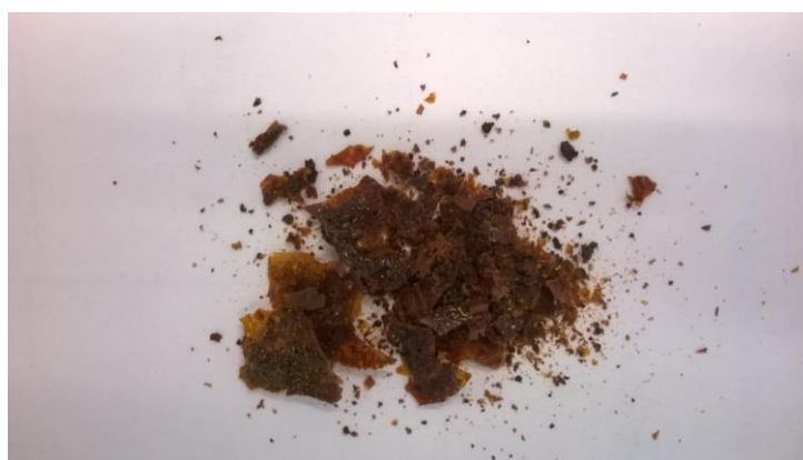
Figure 3.41: Sample of clinoptilolite after pre-treatment with citric acid.
