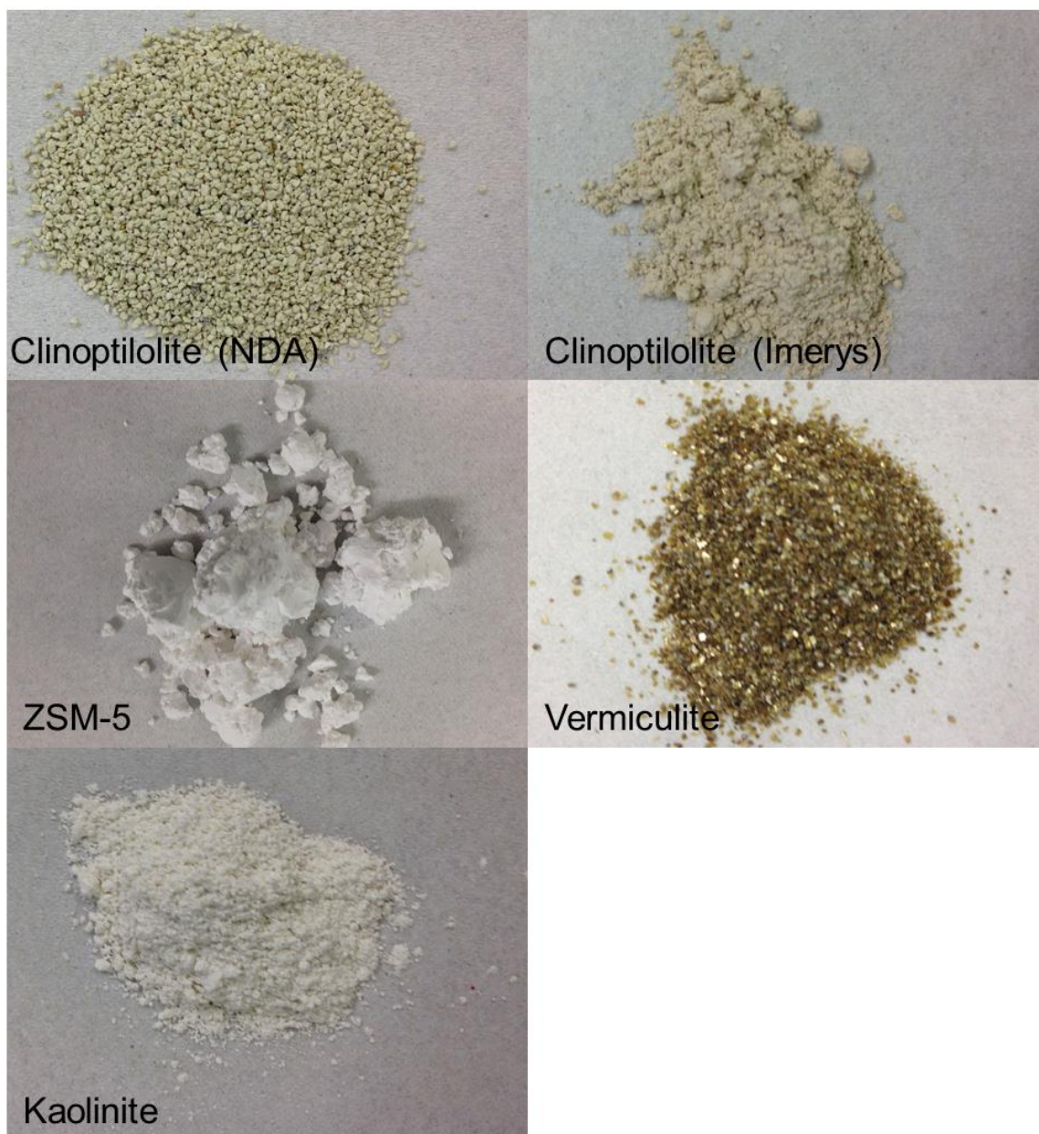
Figure 3.8: Images of the materials selected for grafting experiments.
