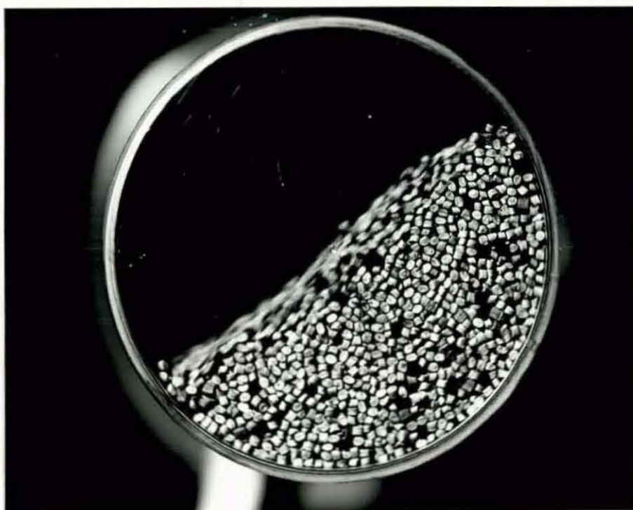
PHOTO 3.6. THE MOTION OF PARTICLES IN THE ROTATING DRUM AT 20rpm (STILL PHOTOGRAPH)
