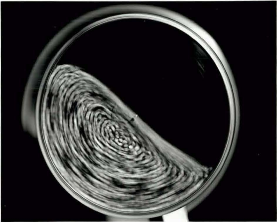
PHOTO 3.8. THE MOTION OF PARTICLES IN THE ROTATING DRUM AT 20rpm (STILL PHOTOGRAPH 1/10 SEC. EXPOSURE TIME)
