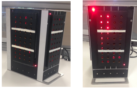
Figure D.1. Photos of synchronising test devise with two four-channel light faces.
