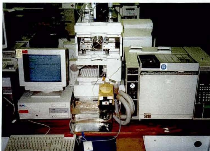
Figure 78: Superheated water chromatograph from left to right: Computer running Chemstation software, 1100 series Hewlett Packard liquid chromatograph, Hewlett Packard 5890 series gas chromatograph, front: water tank with Techne TE-8A thermostat connected to water jacket.
