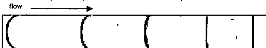
Figure 3: Band broadening in separation column due to frictional heating. A: mobile phase temperature is equilibrated to the column wall temperature. The centre of the column is at a higher temperature than the wall region due to the frictional heating and poor heat transfer in the packed column. B: mobile phase temperature is below column wall temperature. The centre of the column is cooler than the wall region. The temperature in the centre catches up with wall region due to frictional heating.
