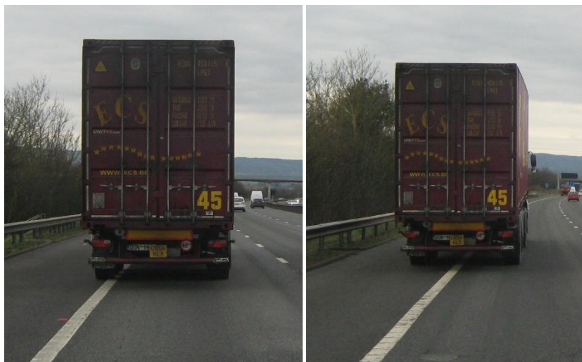
Figure 1. Hard-shoulder incursion of a truck on the motorway (slight/serious). (Source: P. Michalaki)
