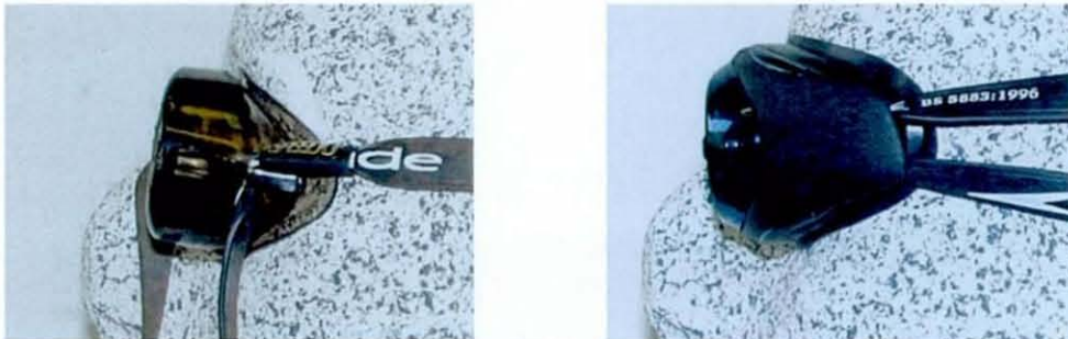
Figure 3.1, Pictures of the Speedo Aquablade (left) and Airframe (right) showing variances in profile. It can easily be seen from Figure 3.1 that the footprint of the seal has been only slightly increased in the Airframe, with the most notable difference being the amount the goggle protrudes from the face. Once again, this illustrates that even at the extreme ends of goggle design, the seal footprint varies only a relatively small amount.
