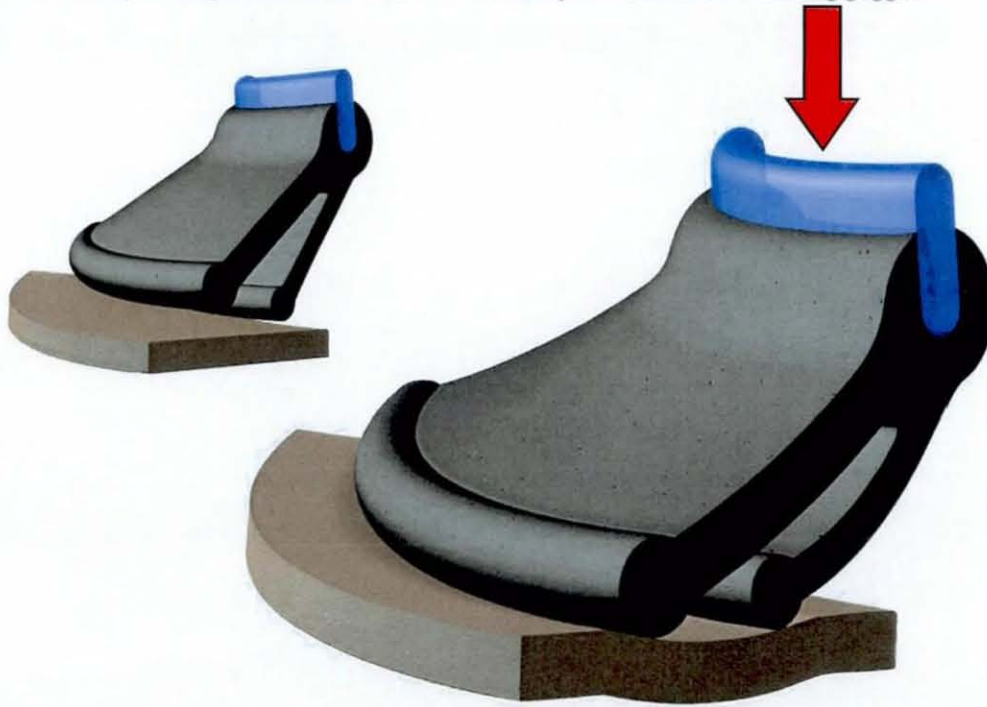
Figure 7.15, Compression of seal
