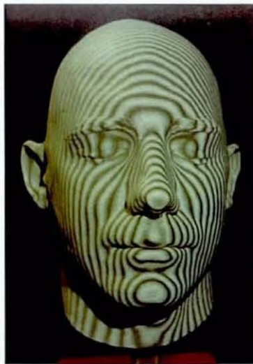
Figure 5.14, Moiré fringe contours being projected on a surface
