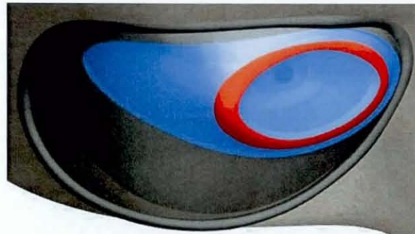
Figure 7.35, Blended corner radius of flat lens section
