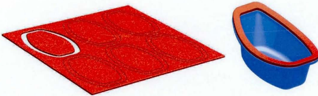
Figure 4.3, Process of using sheet foam to cut seal shapes
