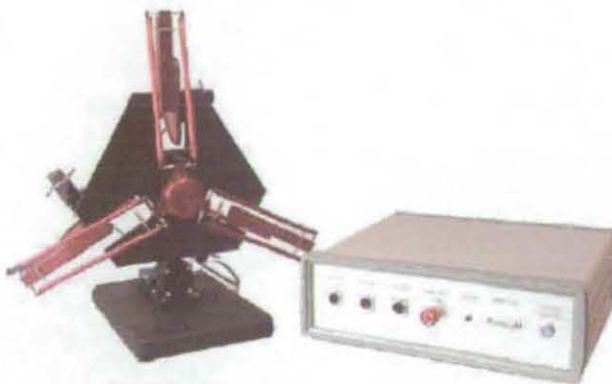
Figure 32: Impedance haptic device: The Delta haptic device
