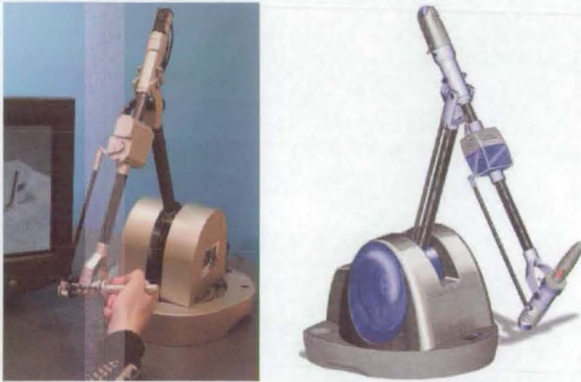
Figure 33: Impedance haptic device: The Virtuose haptic device
