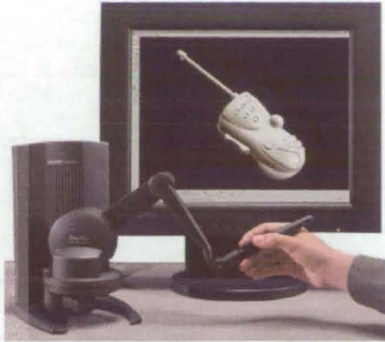
Figure 31: Impedance haptic device: The Phantom haptic device
