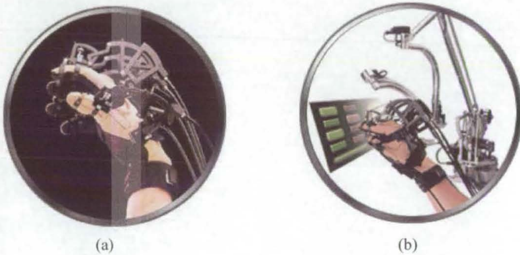
Figure 35: The CyberGrasp and CyberForce system
