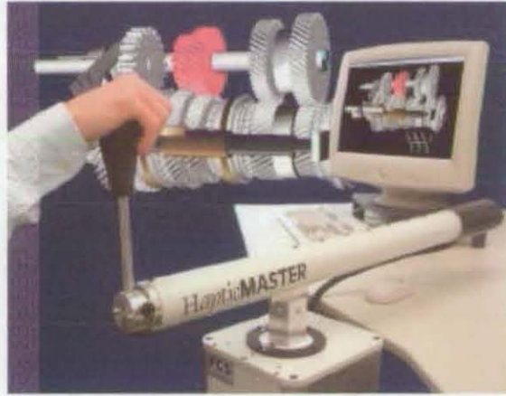
Figure 34: The FCS Haptic Master used in a gear shift simulator
