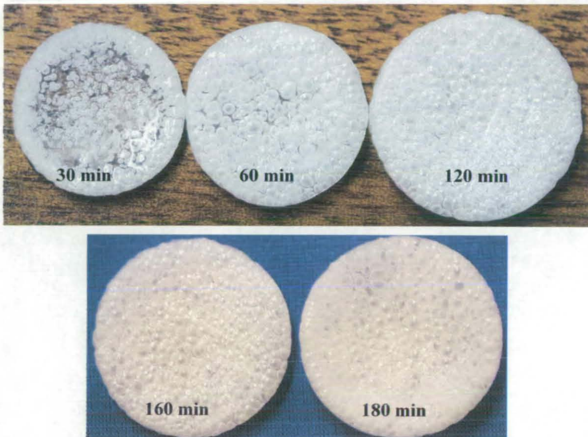
Figure 6 - 16 : Photographs of samples of PS depressurised after holding for different times (30 to 120 min) at 100 °C and 54 bar (1 mm thick x 20 mm diameter).
