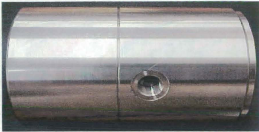
Figure 3 - 23: High pressure view cell.
