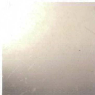
Figure 6 - 29: Photograph of a 1 mm thick PS sample at various times after the onset of depressurisation after holding at 44 bar (in CO 2 ) and 70 °C for 2 hours. No bubbles are seen in any of the images. This photo has been taken at 600 sec and 0 bar (scale of images is 6 x 6 mm).
