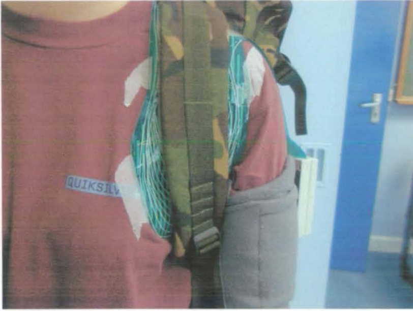
Fig 5.2 : Placement of Backpack over Pressure Sensor
