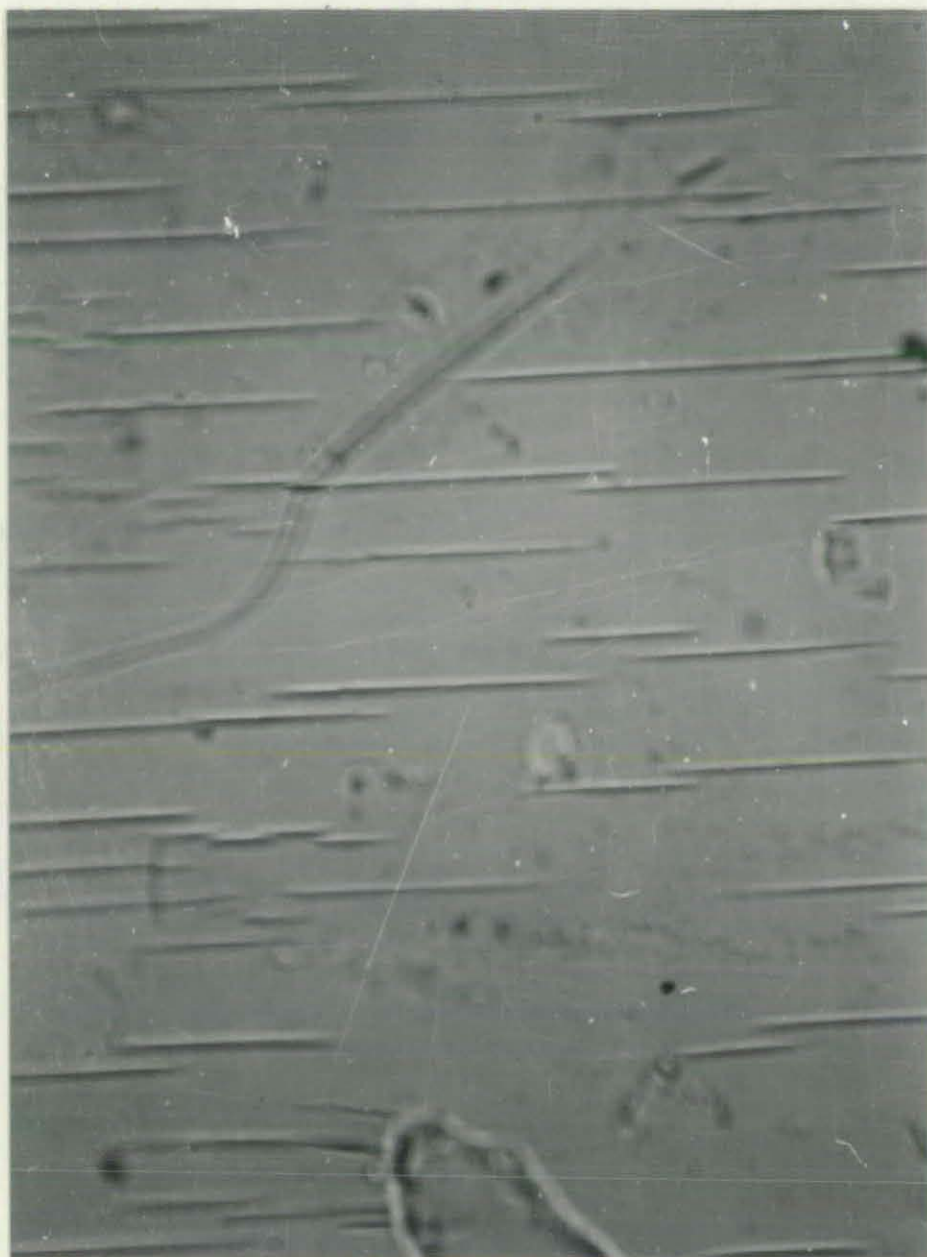
Fig. 5.10(a) UPVC Surface Crazing (X150). After recovery from a tensile stress of 40 \text{ MN/m}^2 at 20^\circ\text{C}
