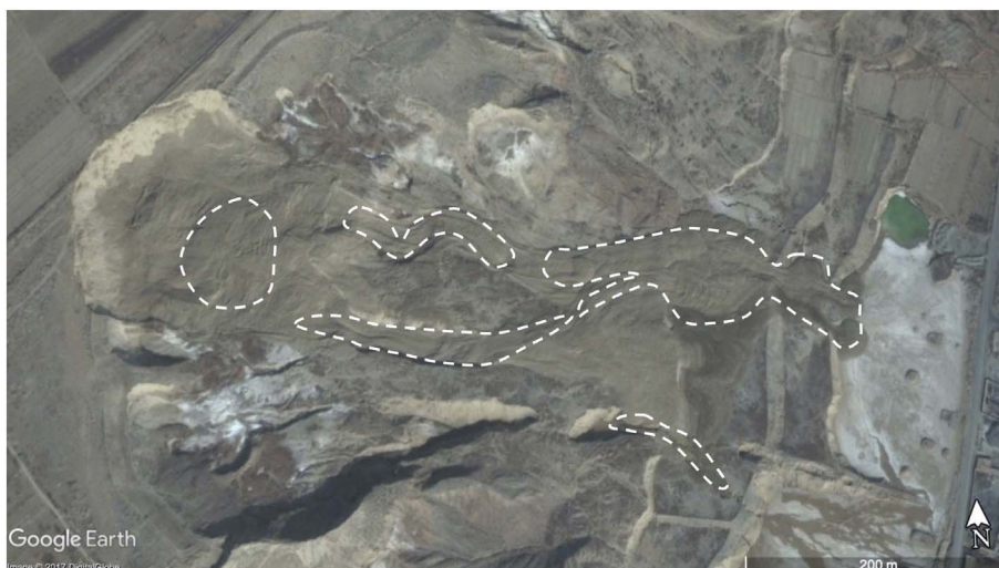
Fig. 11. Post-event satellite image of the Heifangtai 2015 landslide site, with main deposit areas enclosed by dotted lines. (Image from google.com)
