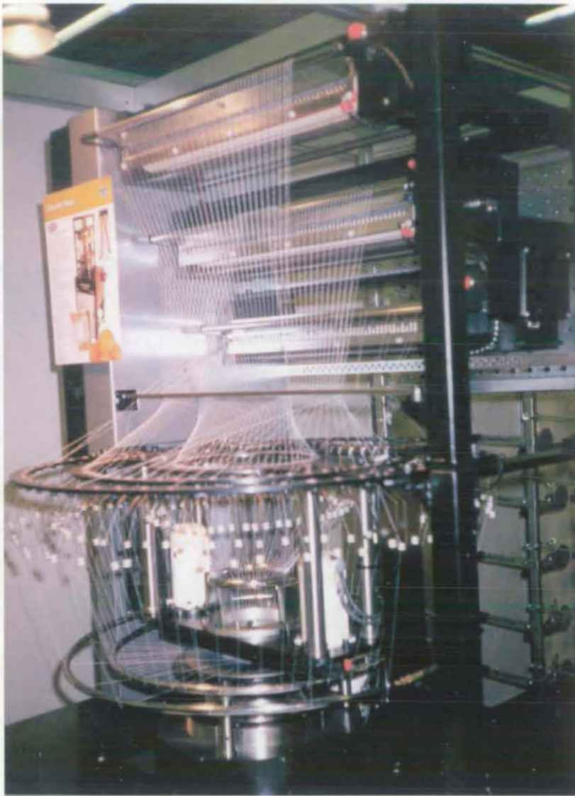
Figure 7-14. Yarn Paths from Let-off Units to Three Rings
