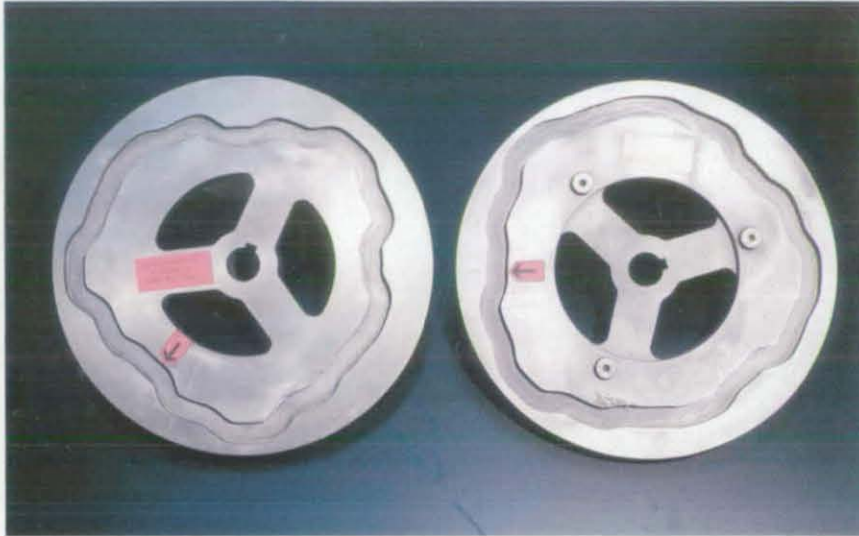
Figure 7-3. Cams for 8-course Patterns.
