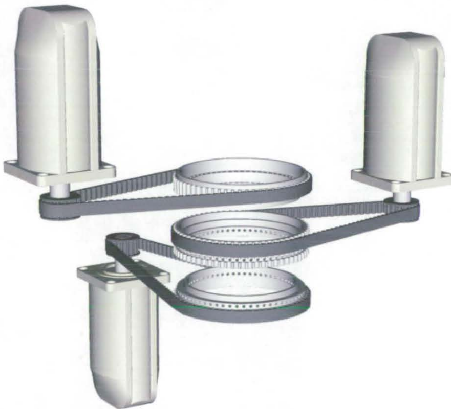
Figure 7-16. Servomotor Controlled Patterning Mechanism.
