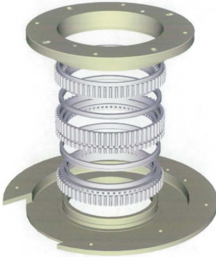
Figure 7-15. Exploded Patterning Rings Assembly
