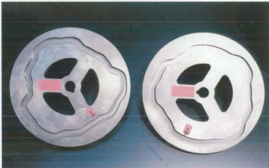
Figure 7-4. Cams for 6-course Patterns
