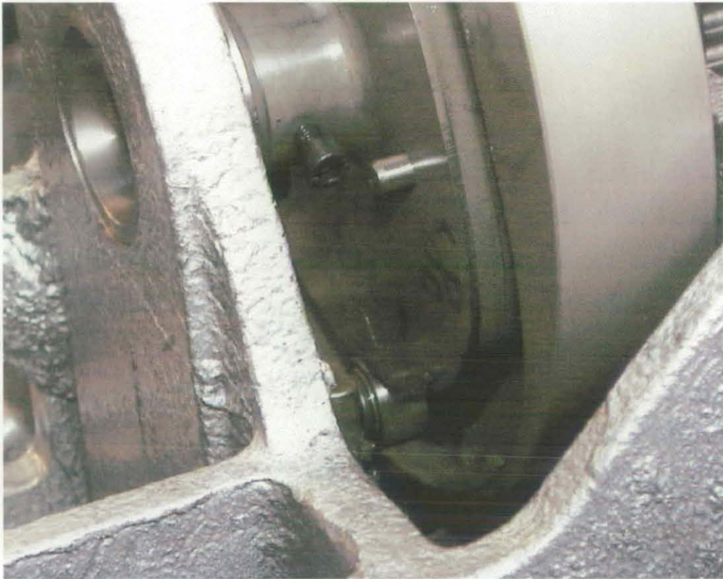
Figure 5-5. Detail of Roller Follower in Cam Track
