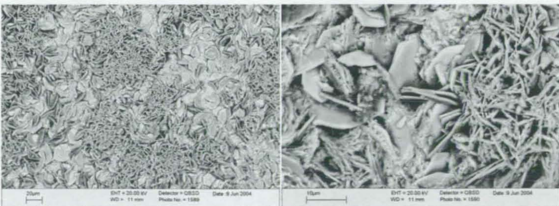
Fig. 6-102 Microstructure of the corrosion products on Sn-Ag-Cu solder after the test with scanning rate 30 mV/min.
