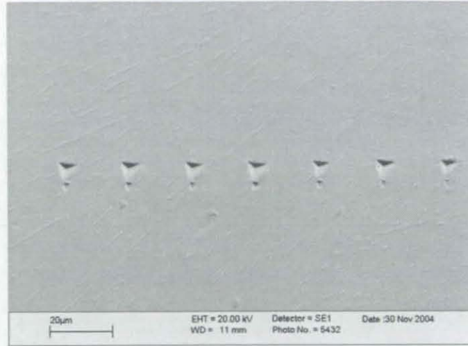
Fig. 6-64 Indentations on Sn-Ag solder in a Sn-Ag/EN solder joint.
