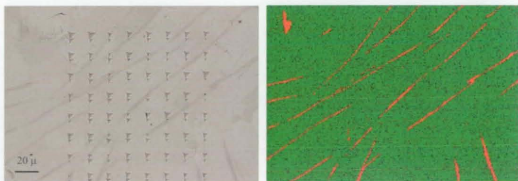
Fig. 6-70 Indentations and element mapping in Sn-Ag bulk solder cooled in furnace. Element mapping, red: Ag, green: Sn.
