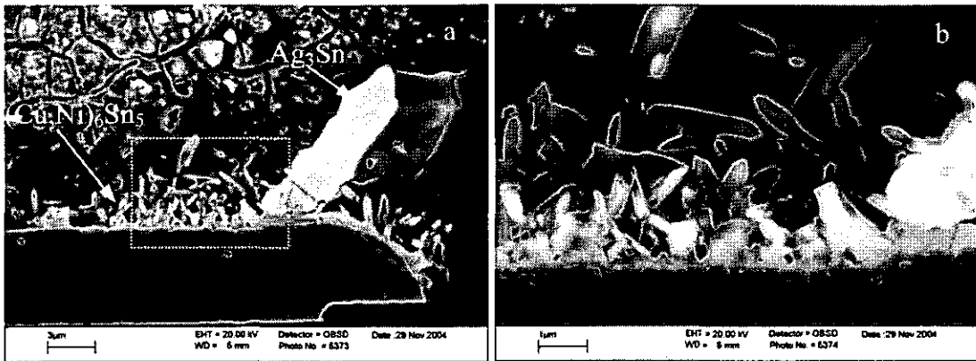
Fig. 6-29 Morphologies of (\text{Cu,Ni})_6\text{Sn}_5 and \text{Ag}_3\text{Sn} IMCs in Sn-Ag-Cu solder bumps.
