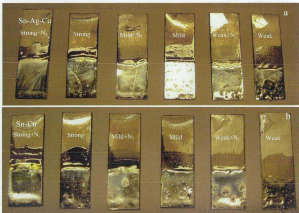
Fig. 7-3 EN plated samples after the wettability tests in Sn-Ag-Cu and Sn-Cu solders.
