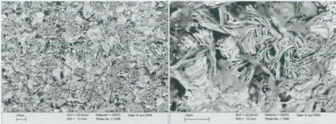
Fig. 6-100 Microstructure of the corrosion products on Sn-Ag solder after the test with scanning rate 30 mV/min.
