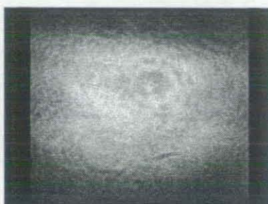
Fig. 3.12: Interference between +1 and 0 order beams—no fringes visible due to inherent high-speed temporal phase modulation.
