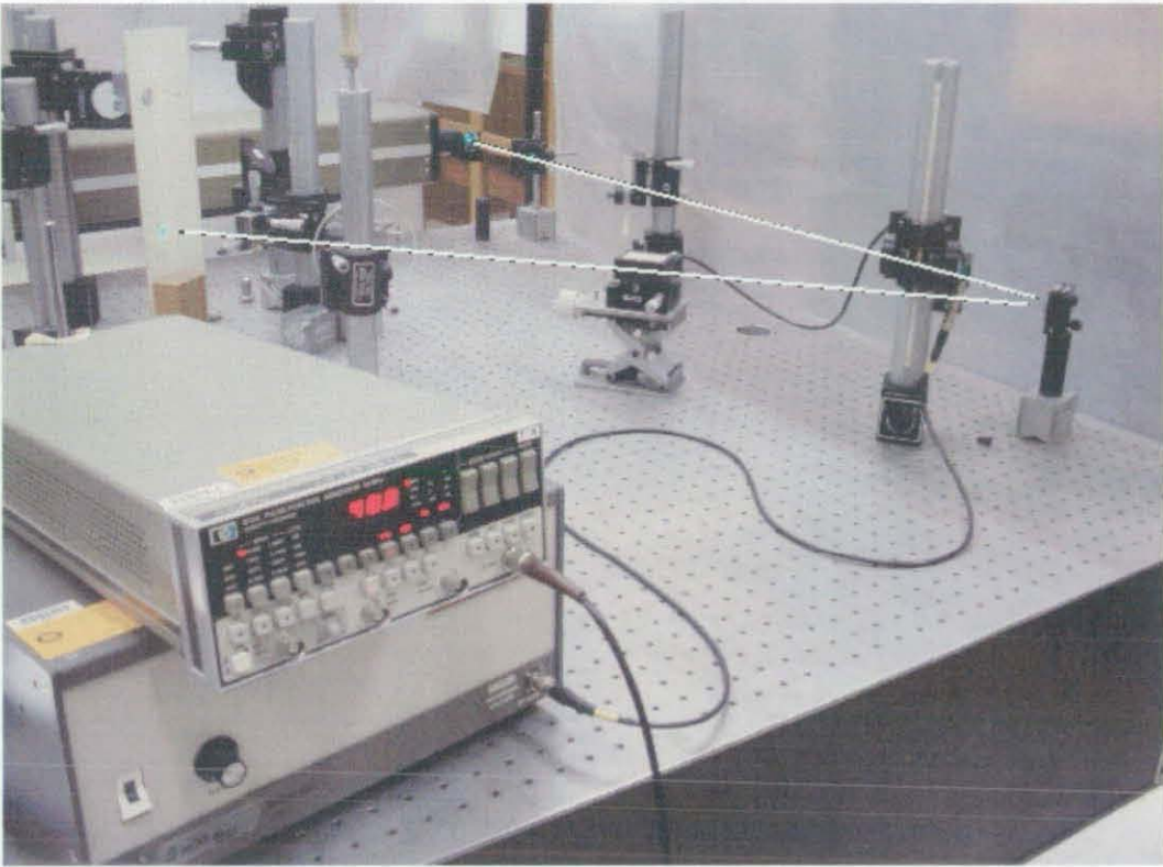
Fig. 3.11: Experimental system with dual AOD's; laser path highlighted.
