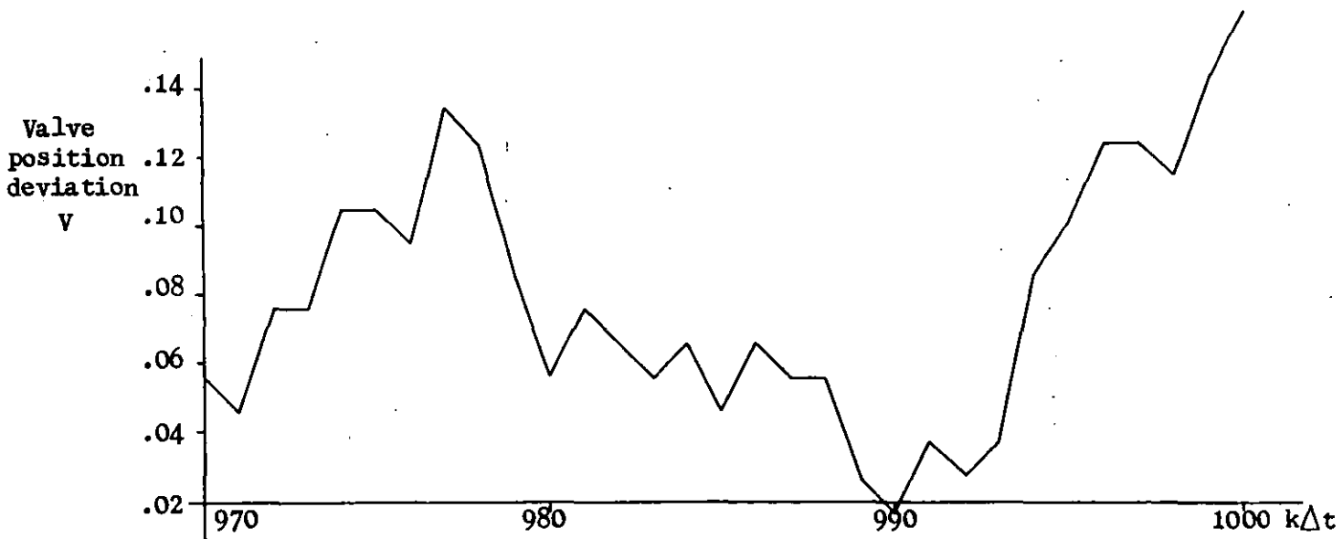
FIGURE 3.17c Valve position deviation measurement in analogue setpoint control experiments.
