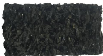
Figure 1. Regupol 6010 SP shockpad disc specimen used for test condition A.
