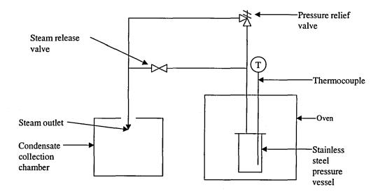
Figure 3.6. Steam Explosion Experimental Equipment.
