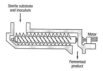
Figure 2.24 Continuous Screw Bioreactor (Chisti, 1999)
