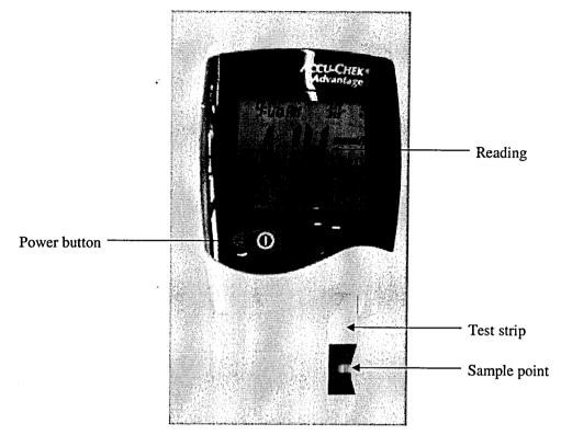
Figure 3.12. Accu-chek Advantage II Glucose Detector.
