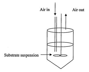
Figure 2.23 Agitated Batch Reactor.
