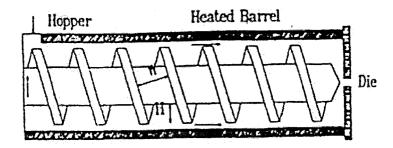
Figure 2.17 Diagram of a Single Screw Extruder (Jaluria and Wang, 1999).
