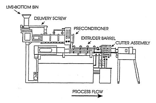
Figure 2.18 Flow Diagram of an Extruder (Brent, 1999).
