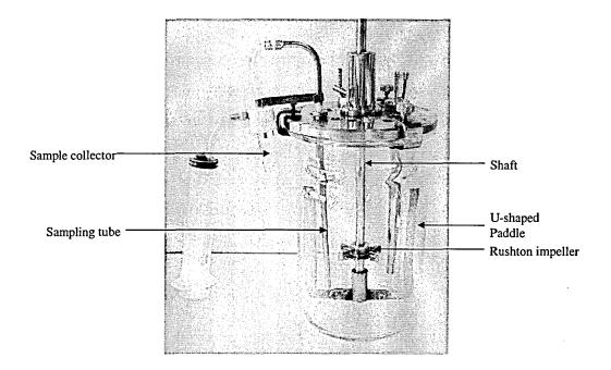
Figure 3.14. Glass Bioreactor.
