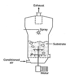
Figure 2.21 A Fluidized Bed Bioreactor (Chisti, 1999).
