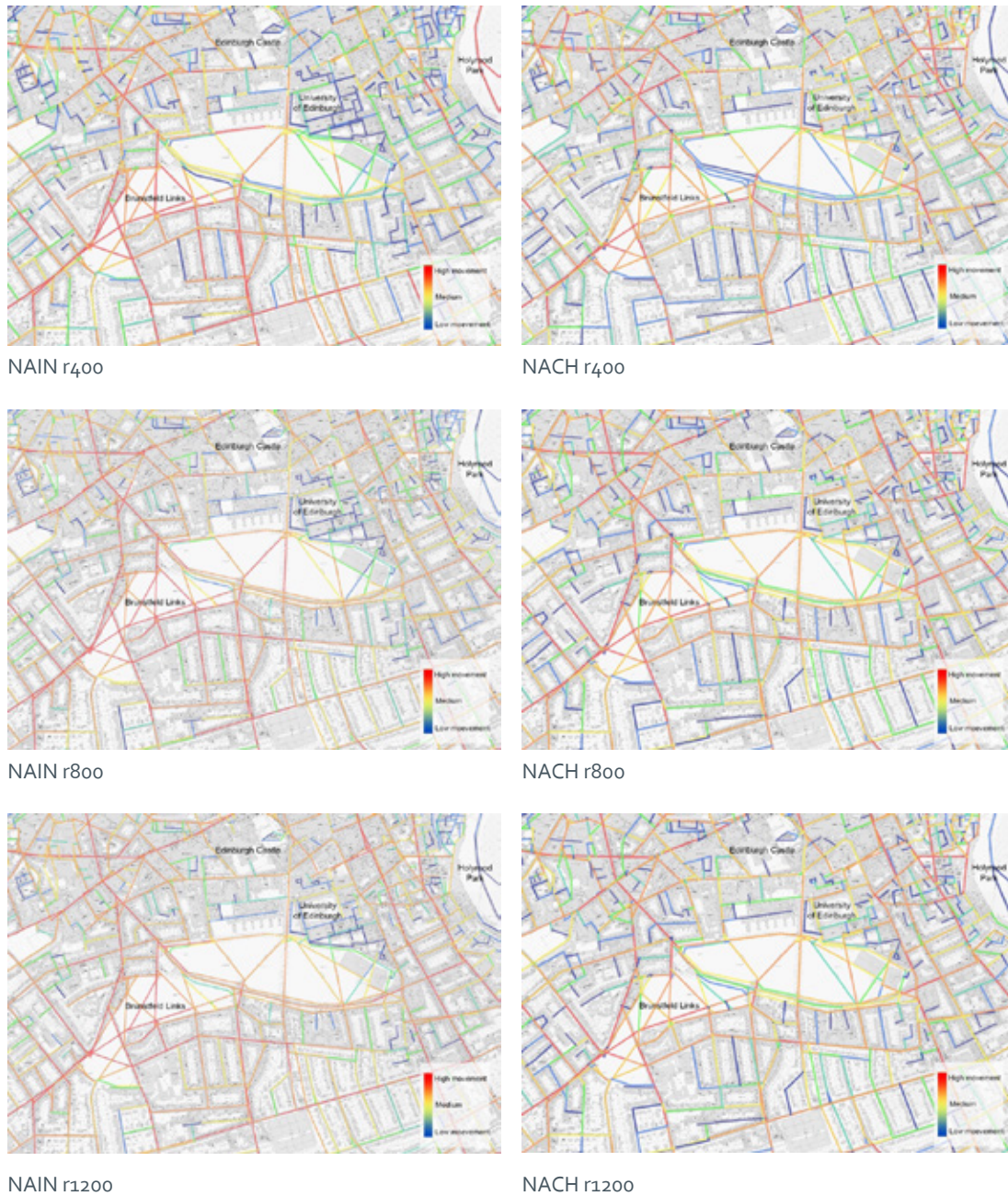
Figure 2 - Analysis of NAIN and NACH measurements using the Depthmap software. Source: EDINA Digimap (background) and Space Syntax Limited (segment map).
