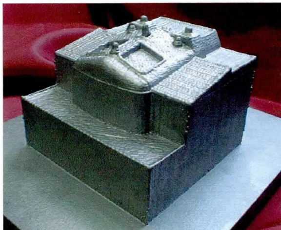
Figure 2.7: Injection moulding tool by LENS process [37]
