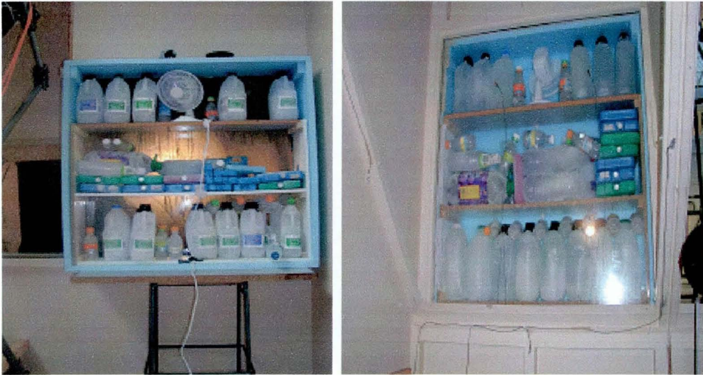
Figure 4.25, The insulated box used to simulate cold external environmental conditions., viewed from inside and outside the chamber
