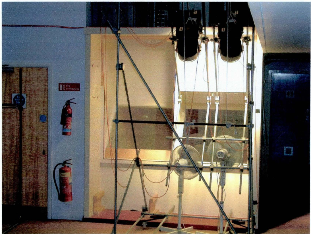
Figure 2.4, Solar simulation chamber with external lamp rig
