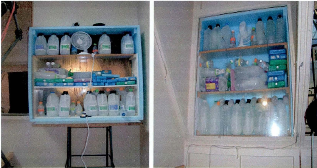
Figure 2.5, The insulated box used to simulate cold external environmental conditions. view from inside and outside
