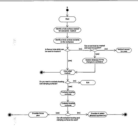
Figure 6.12 - Check the Applicability of Concentric Method in UML Activity Diagram for Support Process Planning Application
