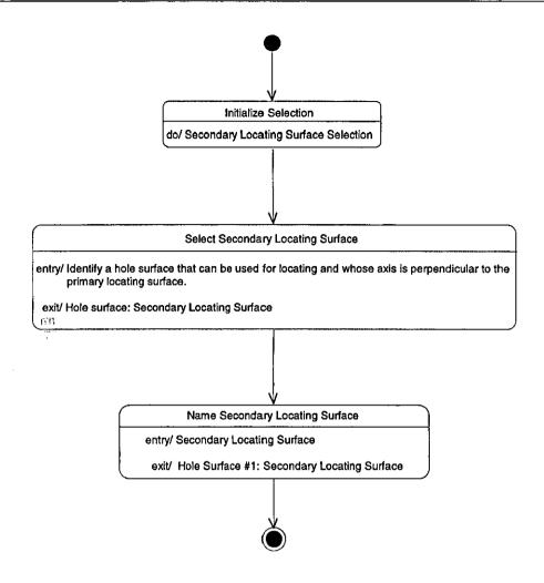
Figure 5.32 - Secondary Locating Surface Selection for Radial Method
