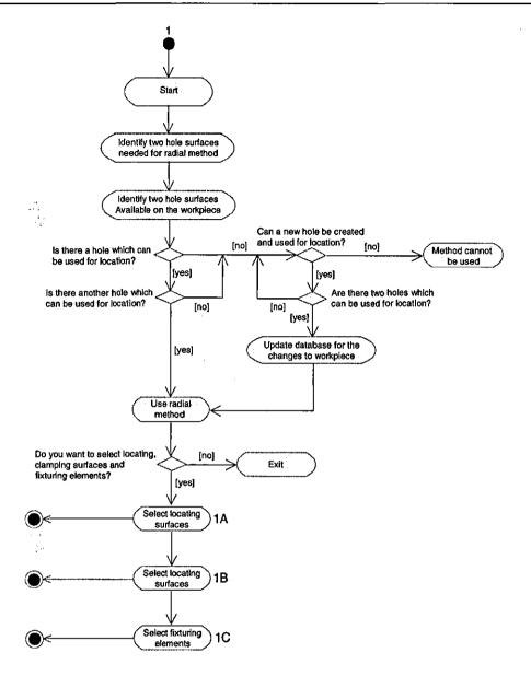
Figure 6.16 - Check the Applicability of Radial Method in UML Activity Diagram for Support Fixture Planning Application
