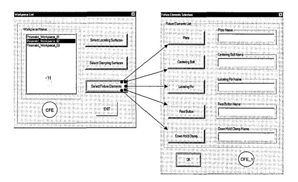
Figure 7.25 – The Dialogs for Selecting Fixture Elements to Support Fixture Planning Using the Concentric Method
