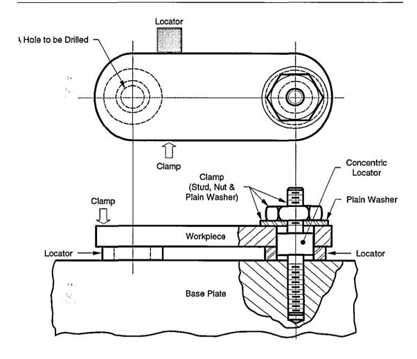
Figure 5.15 - The Clamping for Concentric Method
