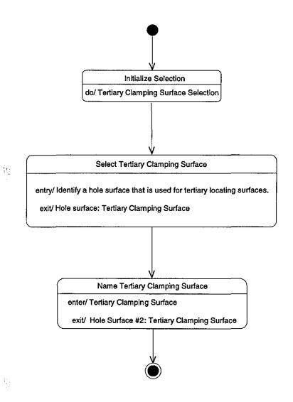
Figure 5.43- Tertiary Clamping Surface Selection for Radial Method
