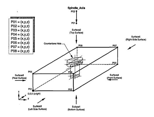
Figure 5.24 – Example of a Prismatic Workpiece as Depicted in the Product Model
