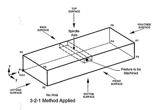
LOCATING SURFACES: Primary Locating Surface **BOTTOM SURFACE** Secondary Locating Surface BACK\_SURFACE **Tertiary Locating Surface** RIGHTSIDE\_SURFACE **CLAMPING SURFACES:** Primary Clamping Surface TOP\_SURFACE Secondary Clamping Surface FRONT SURFACE **Tertiary Clamping Surface** LEFTSIDE\_SURFACE MODULAR FIXTURING ELEMENTS: Base Plate BASEPLATE\_REF# **Rest Buttons** RESTBUTTONS\_REF# Locating Pins LOCATINGPIN\_REF# Clamp Element CLAMPELEMENT\_REF#
