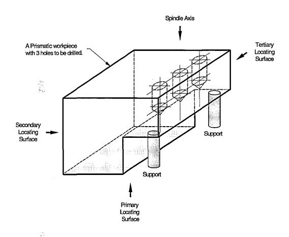
Figure 5.6 - A Prismatic Workpiece with Three Blind Holes Using 3-2-1 Locating Method
