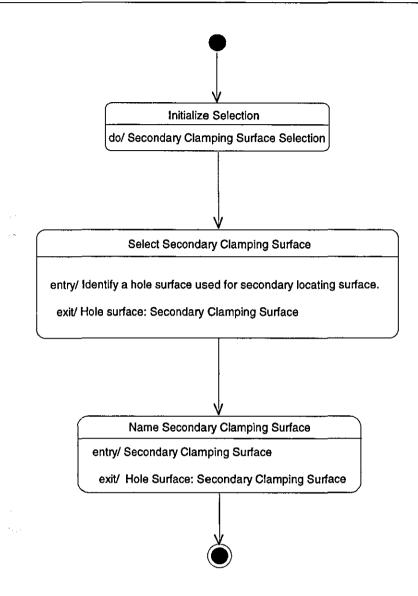
Figure 5.39 - Secondary Clamping Surface Selection for Concentric Method
