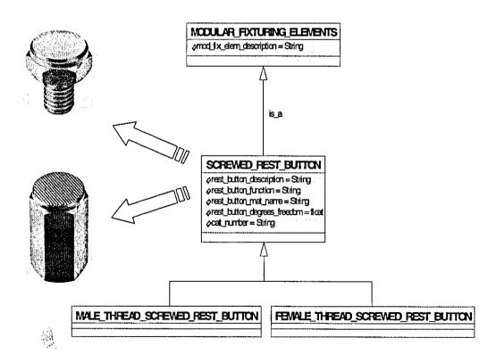
Figure 5.47 – The Representation of Screwed Rest Buttons
