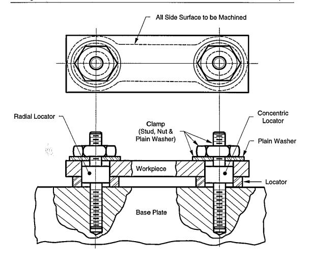
Figure 5.16 - The Clamping for Radial Method
