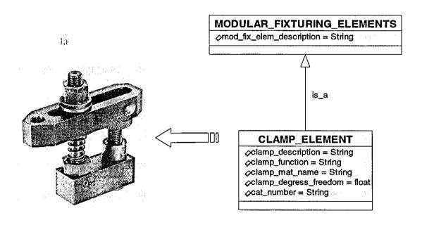
Figure 5.48 - The Representation of Clamp Elements
