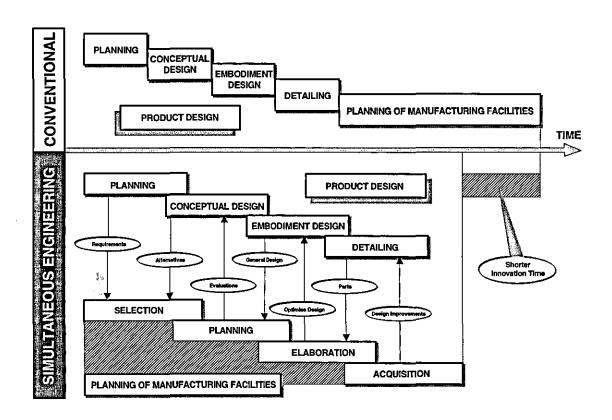
Figure 2.2 – Simultaneous Engineering [Ref: Weck et al., 1991]
