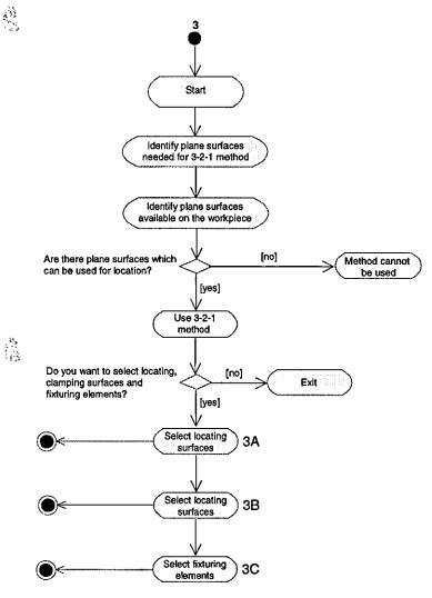
Figure 6.23 - Check the Applicability of 3-2-1 Method in UML Activity Diagram for Support Fixture Planning Application
