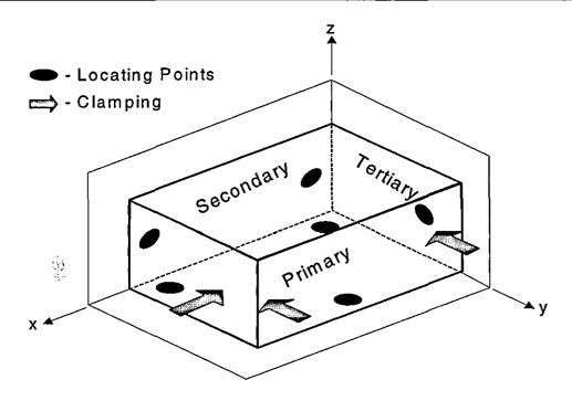
Figure 3.6 – The 3-2-1 Locating Method for a Prismatic Workpiece [Ref: Wilson 1962]
