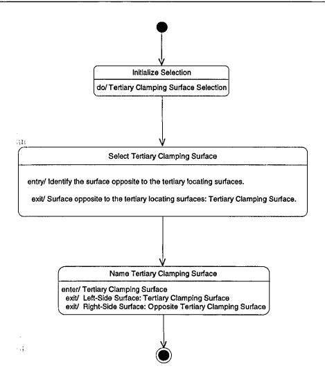
Figure 5.37 - Tertiary Clamping Surface Selection for 3-2-1 Clamping
