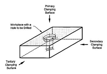
Figure 5.14 - The Clamping for 3-2-1 Method
