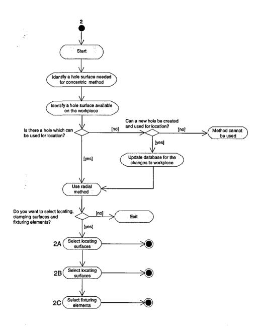
Figure 6.18 — Check the Applicability of Concentric Method in UML Activity Diagram for Support Fixture Planning Application
