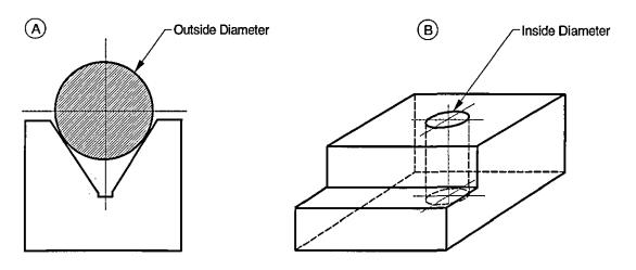
Figure 5.7 – The Concentric Locating Method
