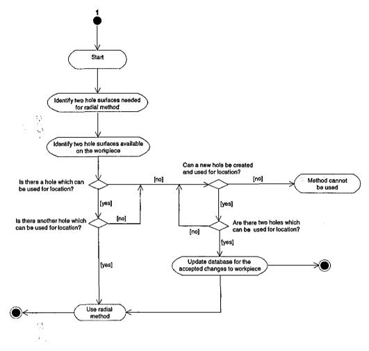
Figure 6.3 - Check the Applicability of Radial Method in UML Activity Diagram for Support Product Design Application
