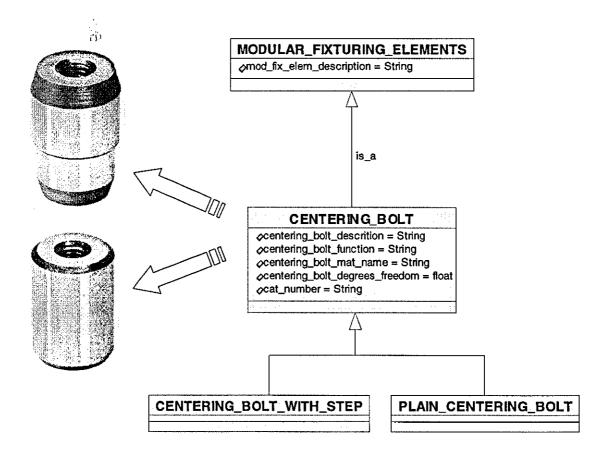
Figure 5.50 – The Representation of Centering Bolts
