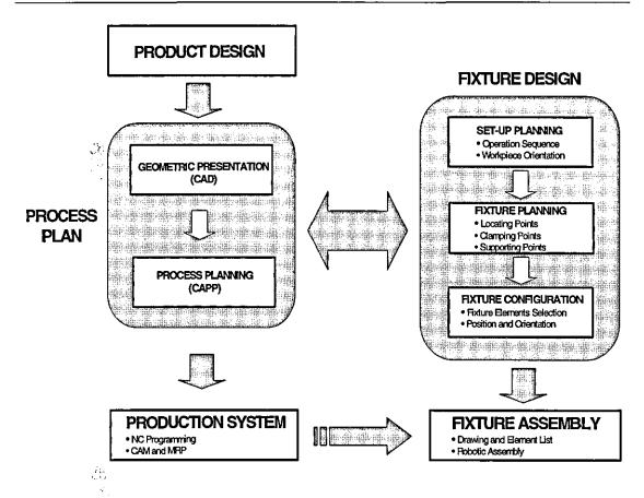
Figure 2.1 - Fixture Design in Manufacturing Systems [Ref: Rong et al., 1995]
