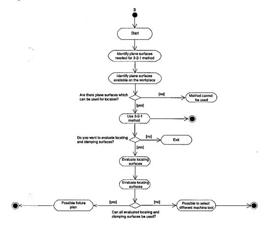
Figure 6.13 - Check the Applicability of 3-2-1 Method in UML Activity Diagram for Support Process Planning Application
