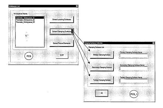
Figure 7.17 – The Dialogs for Selecting Clamping Surfaces to Support Fixture Planning Using the 3-2-1 Method
