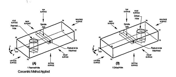
Figure 6.6 - Sample Variations of a Workpiece for the Applicability of Concentric Method
