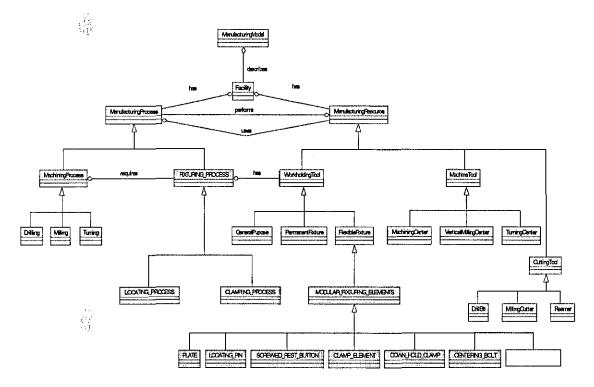
Figure 5.22 – The MOSES Manufacturing Model Structure in UML Class Diagram with the Fixturing Information
