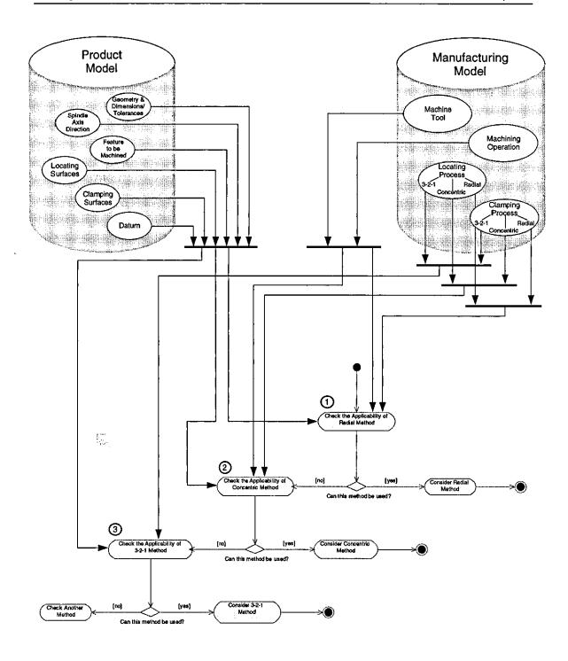
Figure 6.10 - Support Process Planning Activities in UML Activity Diagram
