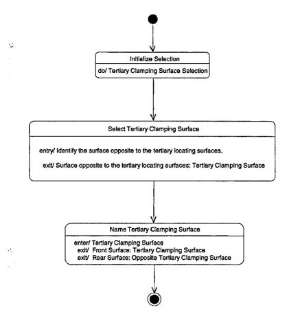
Figure 5.40 – Tertiary Clamping Surface Selection for Concentric Method
