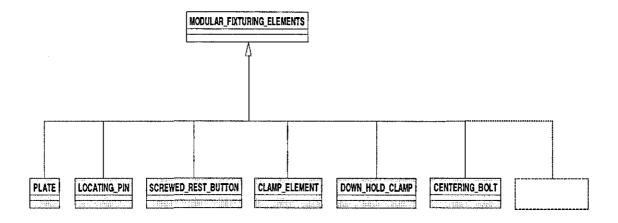
(ii) Figure 5.44 - Fixturing Elements Data Structure in UML Class Diagram
