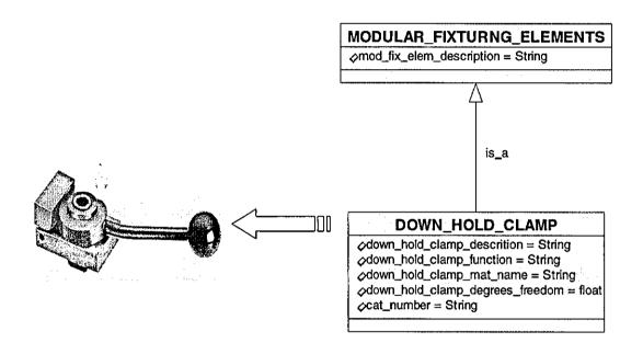
Figure 5.49 – The Representation of Down Hold Clamps
