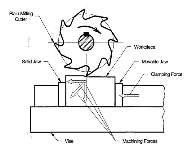
Figure 5.11 - Cutting Forces in a Milling Machine Operation
