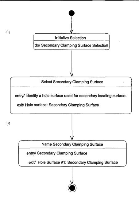
Figure 5.42 - Secondary Clamping Surface Selection for Radial Method
