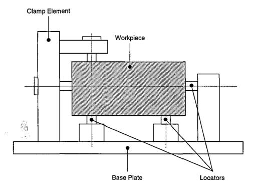
Figure 5.2 - A workpiece being Located and Clamped on a Fixture
