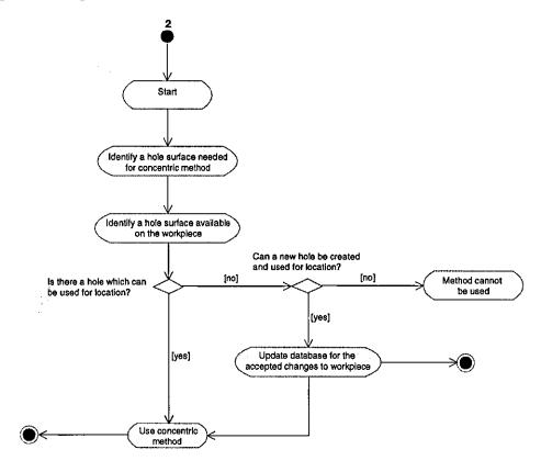
Figure 6.5 — Check the Applicability of Concentric Method in UML Activity Diagram for Support Product Design Application
