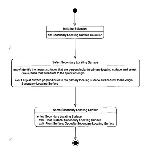
Figure 5.26 - Secondary Locating Surface Selection for 3-2-1 Locating
