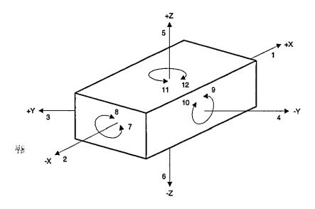
Figure 3.5 – The Degrees of Freedom for a Prismatic Workpiece [Ref: Hoffman 1985]
