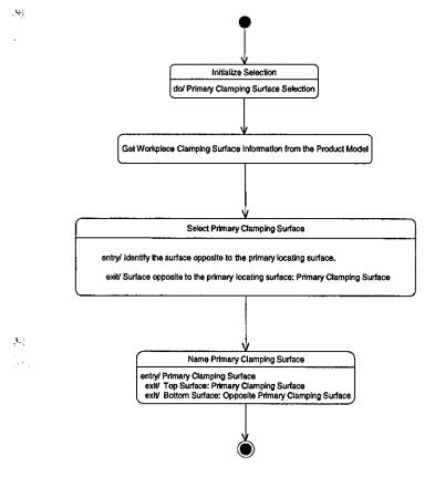
Figure 5.35 – Primary Clamping Surface Selection for 3-2-1 Clamping in UML Activity Diagram
