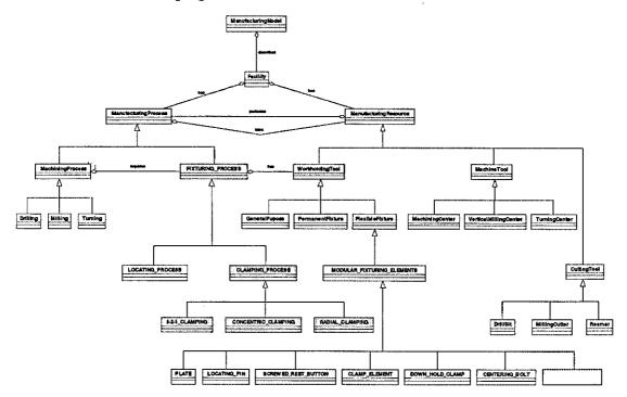
Figure 5.28 - Clamping Process Data Structure in UML Class Diagram
