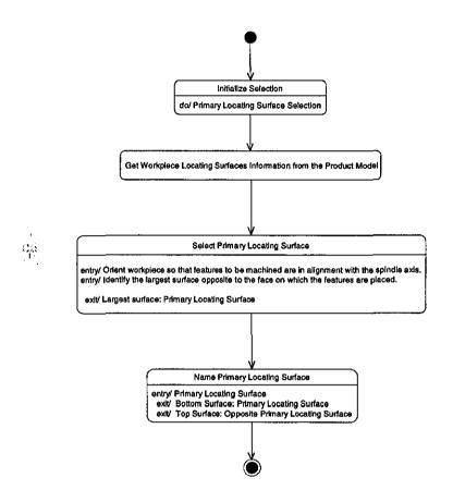
Figure 5.25 – Primary Locating Surface Selection for 3-2-1 Locating in UML Activity Diagram
