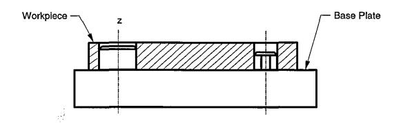
Figure 5.10 – Workpiece Mounted on a Base Plate with Two Locating Pins
