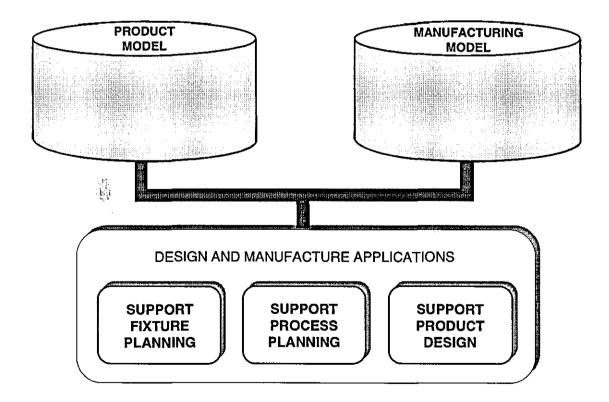
Figure 4.1 – A Fixturing Information Model within the MOSES Concept
