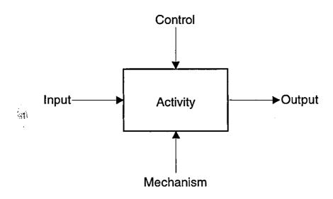
Figure A-A.2 - IDEF0 Function Box and Interface Arrows
