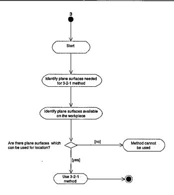
Figure 6.7 - Check the Applicability of 3-2-1 Method in UML Activity Diagram for Support Product Design Application
