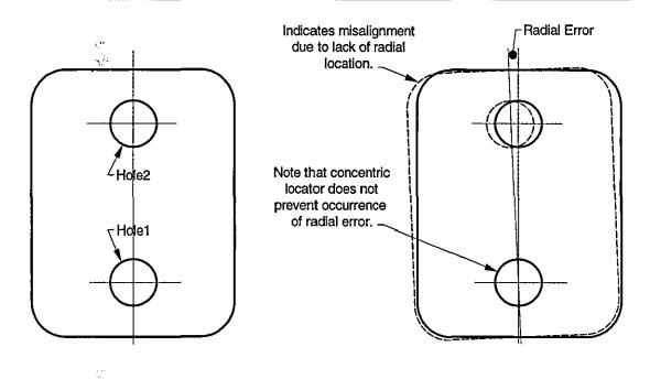
Figure 5.8 – The Radial Locating Method
