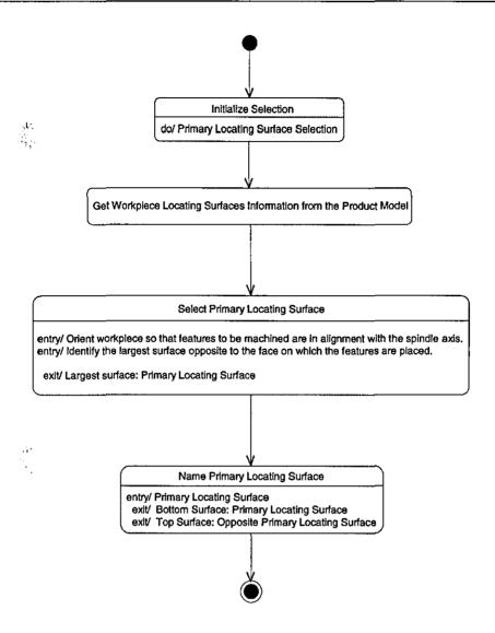
Figure 5.31 – Primary Locating Surface Selection for Radial Method in UML Activity Diagram
