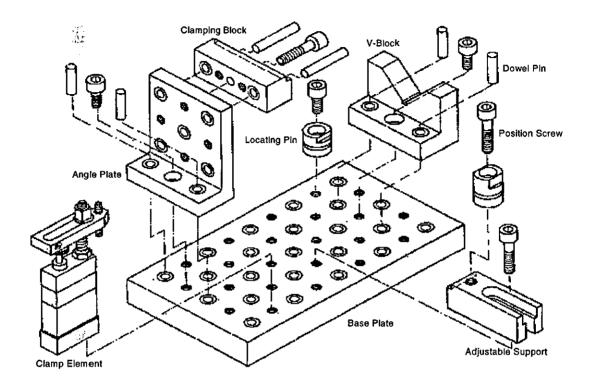
Figure 3.8 – The Modular Fixture Kits [Ref: Rong et al., 1995]
