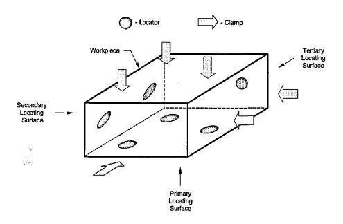
Figure 5.9 - The Clamps are Placed Directly Opposite to the Locators
