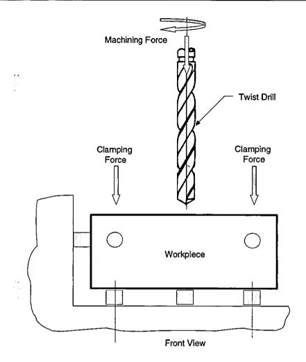
Figure 5.12 - Cutting Forces in a Drilling Operation
