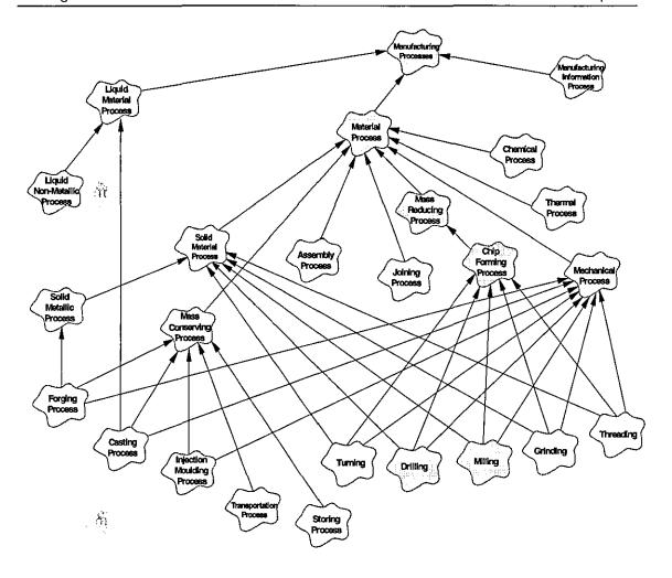
Figure 3.3 – The MOSES Manufacturing Process Representation [Ref: Molina 1995]
