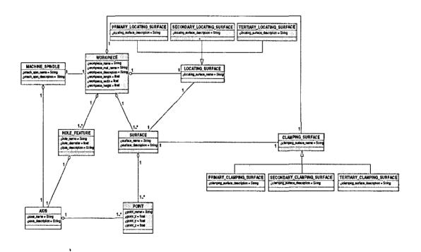
Figure 5.52 - The Structure of the Product Data Model in UML Class Diagram
