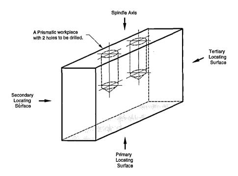
Figure 5.5B - A Prismatic Workpiece with Two Blind Holes Using the 3-2-1 Locating Method
