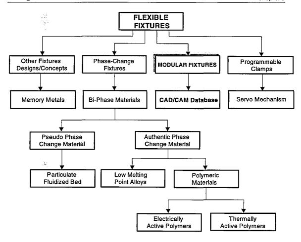
Figure 3.7 – An Overview of Flexible Fixturing Methodologies [Ref: Kumar *et al.*, 1992]
