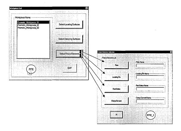
Figure 7.19 – The Dialogs for Selecting Fixture Elements to Support Fixture Planning Using the 3-2-1 Method
