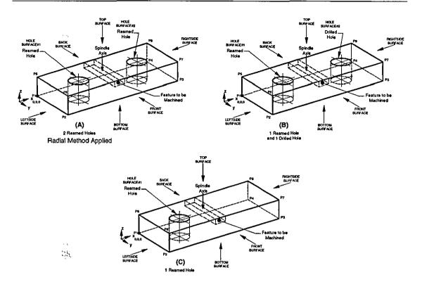
Figure 6.4 - Sample Variations on a Workpiece for the Applicability of Radial Method
