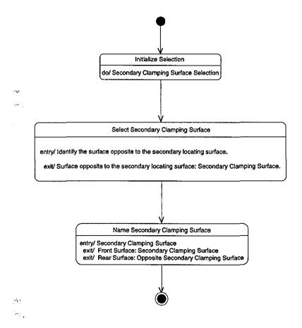
Figure 5.36- Secondary Clamping Surface Selection for 3-2-1 Clamping
