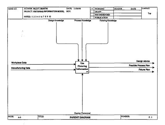
Figure 5.17 - The Parent Diagram for Use Fixturing Information Activity
