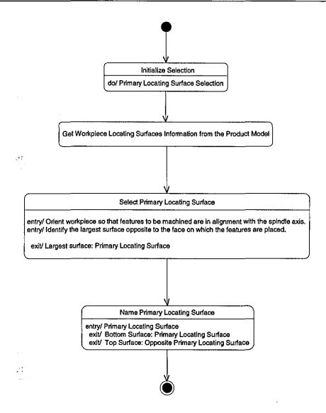
Figure 5.28 – Primary Locating Surface Selection for Concentric Method in UML Activity Diagram
